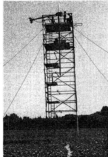
Photo 1. The tower (12 m high) used to perform the reflectance measurements
