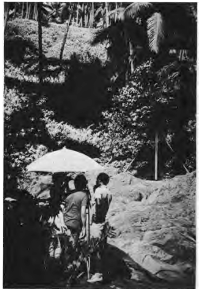
FIGURE 13.5 Dry tilt measurements being made on St. Vincent in March 1977, more than 2 yr before the 1979 eruption. Data obtained from this station helped confirm that the volcano was inflating.
