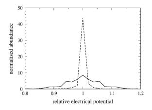
Fig. 1. Histograms of the relative variations of the electrical potential measured for: (1) multiple direct and reciprocal electrode arrangements (dashed line), and (2) random perturbations of the electrode positions (solid line). The relative variations account for the huge range spanned by the potential values (i.e. up to 5 orders of magnitude) and are obtained by dividing each measurement by the average potential corresponding to a given electrode quadrupole.
