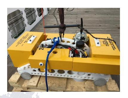
The specific construction of ballast releasing mechanism has a tendency to fail. In viscous environments OBS gets suck and recovery fails.
