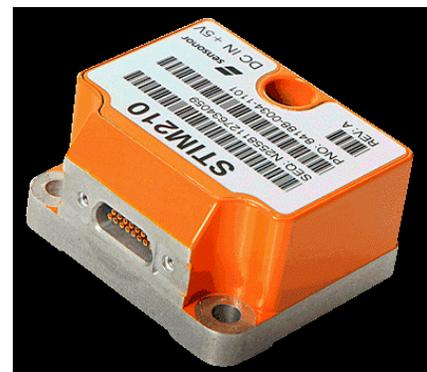
Figure 2: Picture of the Sensoror STIM210 MEMS Gyroscope package
