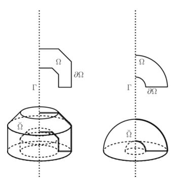
Figure 1. The approach we describe aims primarily at solving the Navier–Stokes equation in spherical/spheroidal shells (right). Its flexibility allows, however, to handle axisymmetric containers of more complicated shape (left) that one could use in a laboratory experiment. In each case, the 3-D domain  $\check{\Omega}$  follows from the revolution of its meridional section  $\Omega$  around its axis of symmetry  $\Gamma$ .  $\partial \Omega$  is the boundary of  $\Omega$ .
