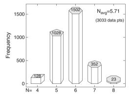
**Fig.** 7 Distribution of the order of the polygonal column cross sections N at all columnar jointing sites combined (3,033 columns). Hexagonal sections are the most frequent (every second) followed by pentagons (every third). The average order of polygons is 5.71
