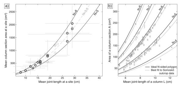
Fig. 9 a Relation of the mean side length La to the mean section area A at columnar jointed igneous rock sites. Dashed grey circles stand for sites with less than 30 area measurements, solid black circles stand for sites with more than 30 area measurements, with grey lines showing the  $1\sigma$  variation of both La and A. Parabolae show the theoretical curves for regular hexagons and pentagons based on Eq. 3. **b** Relation
