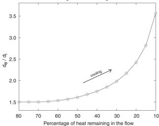
Fig. 12 Thickness ratio of igneous bodies having the same cooling rate, as a function of the remaining heat within the body. See text for details
