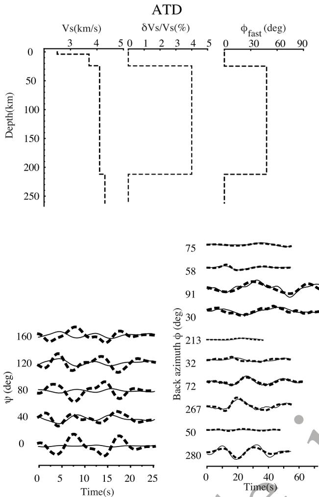
**Figure 9.** Single-layer anisotropic model for station ATD. The anisotropic parameters are  $\phi_{fast} = 43^\circ$  and  $\delta t = 1.6s$  and were taken from *Barruol and Hoffmann* [1999]. The delay time is converted to thickness supposing 4% of anisotropy.
