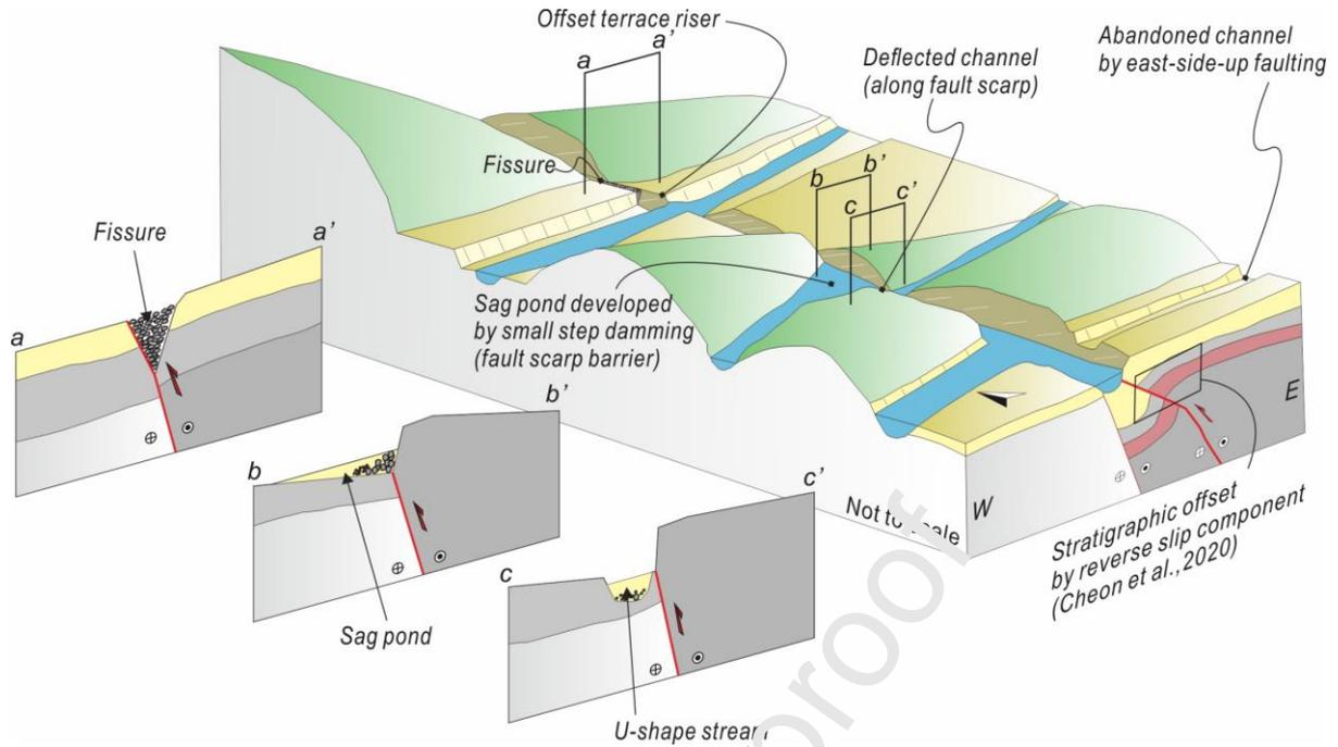
Fig. 9. Schematic diagrams showing landforms and stratigraphic features associated with strike-slip ruptures. A fissure-filling deposit is observed in the WS trench (profile a–a'). A sag pond deposit developed by fault scarp damming is observed in the northern wall of the MH trench (b–b'). A U-shaped cut-and-fill deposit along the fault splay is observed in the southern wall of the MH trench (c–c' profile).
