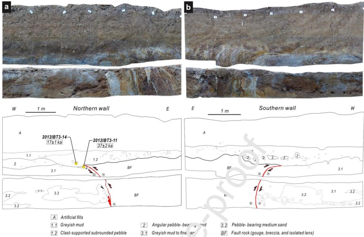
Fig. 8. Photographs and detailed sketches of the northern (a) and southern (b) walls of the IBN trench. The grid interval is 1 m × 1 m. Yellow circles indicate OSL sampling points with ages.
