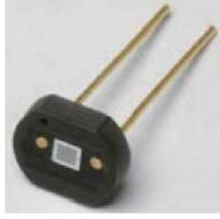
Figure 6: Picture of a ceramic packaged MPPC.
