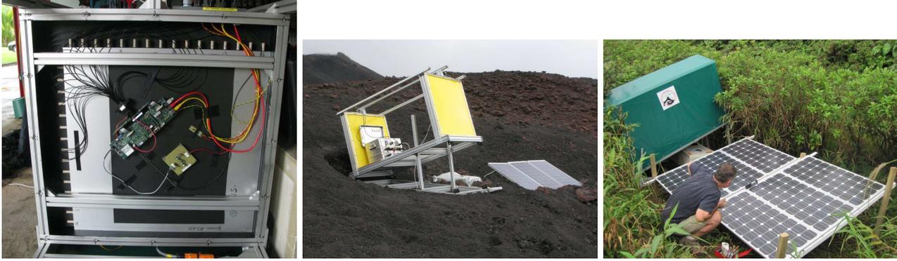
Figure 10: Left: matrix with open case. Middle: complete telescope at the summit of Mount Etna in Sicily. The dip is  $30^\circ$  and the distance between the two matrices is of 115 cm. Solar conditions there allow single solar unit use. Right: telescope covered with its tarpaulin on La Soufrière of Guadeloupe. Two solar units of 270 W each are mandatory because of cloudy weather.
