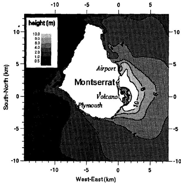
**Fig. 5.** Maximum computed water surface elevation reached during the tsunami propagation. The volcano is indicated by a star, the landslide is assumed to flow down Eastwards.
