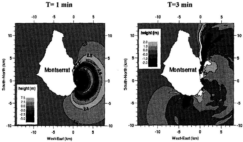
**Fig. 4.** Computed water waves 1 and 3 minutes after the wave generation. The grid increment is 100 meters. These maps have been calculated by a shallow water model for a landslide of 80 millions of m<sup>3</sup> flowing down the Tar River valley.
