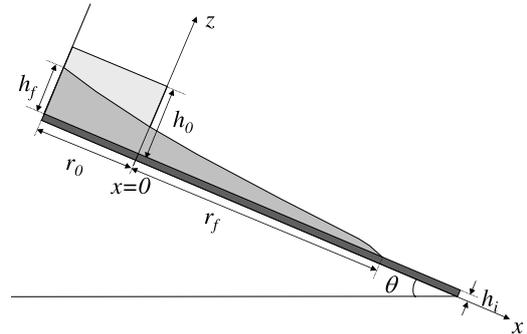
**Figure 4.** Morphometric and control parameters measured in the experiments. The initial mass (light gray) with initial thickness  $h_0 = 14 \text{ cm}$  and radius  $r_0 = 20 \text{ cm}$  (aspect ratio  $a = 0.7$ ) is released on a plane with inclination  $\theta$  covered by an erodible bed of thickness  $h_i$  (dark gray). It forms a deposit (moderate gray) with a length  $r_f$  from  $r_0$ , hereafter called the runout distance, and a final maximum thickness  $h_f$ .
