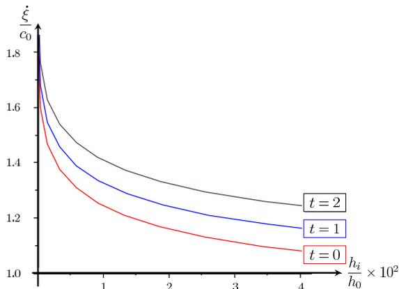
**Figure 23.** Normalized speed of the shock  $\dot{\xi}/c_0$  located at the front of the flow as a function of the normalized thickness of the erodible layer  $h_i/h_0$ , for  $h_0 = 0.14$  m,  $\theta = 22^\circ$ , and  $\theta = 21.5^\circ$ , at different times.
