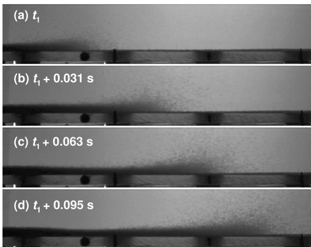
**Figure 21.** Snapshots of the front zone from time  $t_1$  when the front crosses the position  $x = 77 \text{ cm}$  taken every  $0.031 \pm 0.001 \text{ s}$  in the region  $x \in [70, 100] \text{ cm}$  from the gate for granular collapse over a rigid bed ( $h_i = 0 \text{ mm}$ ) at  $\theta = 25.2^\circ$ . The front has a steep shape when saltating grains are not taken into account.
