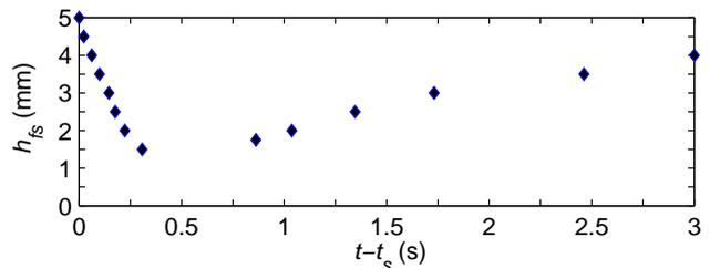
**Figure 18.** Vertical position of the flowing/static interface within the erodible bed  $h_{fs}$  measured at  $x = 90$  cm as a function of time  $t - t_s$ , where  $t_s = 0.6$  s corresponds to the time when the front reaches the position  $x = 90$  cm for the flow at  $\theta = 25.4^\circ$  and  $h_i = 5$  mm (experiment E'25-5).
