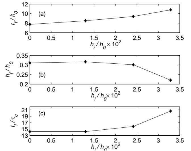
**Figure 12.** Normalized (a) runout distance  $r_f/h_0$ , (b) final thickness at the upper wall  $h_f/h_0$ , and (c) time at which the front stops  $t_f/\tau_c$  where  $\tau_c = \sqrt{h_0/(g \cos \theta)} = 0.124$  s, as a function of the normalized thickness of the erodible bed  $h_i/h_0$  for inclination angle  $\theta = 22^\circ$ .
