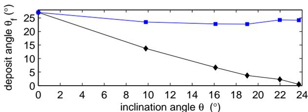
**Figure 8.** The mean angle of the deposit calculated using equation (7) with respect to the inclined plane (diamond) and with respect to the horizontal direction (squares) as a function of the plane inclination  $\theta$ .
