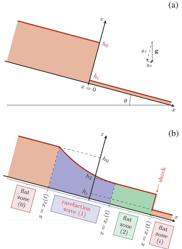
**Figure 22.** Dam-break problem: free surface at (a)  $t = 0$ , and (b)  $t > 0$ .
