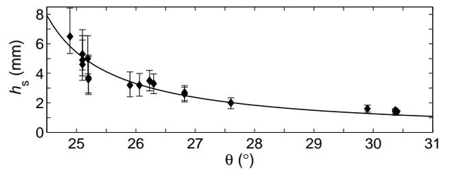
**Figure 5.** The thickness  $h_s$  left on a plane of inclination angle  $\theta$  after steady uniform flows once the supply is cut. The full line is the best fit to the formula (1)  $h_s = \alpha d / (\tan \theta - \tan \delta_1)$  with  $\alpha = 0.26$  and  $\delta_1 = 23.4^\circ$ .
