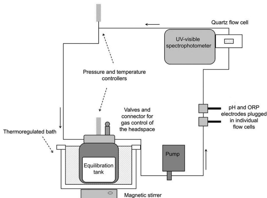
Fig. 1. Schematic description of the biomineralization control cell (BCC) apparatus. Circuit is closed and fluid submitted to an anti-clockwise motion by the pump.
