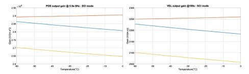
**Fig. 88** SEIS POS output at the Phobos Tide frequency and SEIS VEL output at 100 s, as a function of temperature. Temperature dependency will be recalibrated on Mars but can be considered as linear as a function of frequency and with a frequency dependency as indicated by Fig. 85. The information of temperature dependency will be encrypted in a SEED comment
