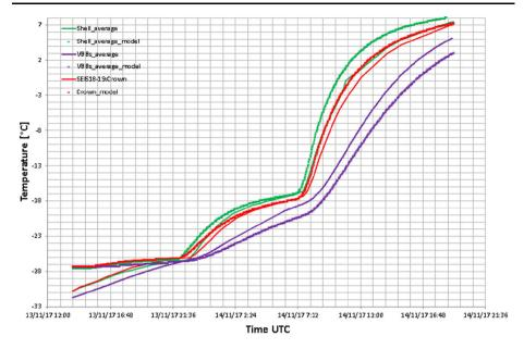
Fig. 111 Comparison model-test data on the warm-up phase of Landed TVAC
