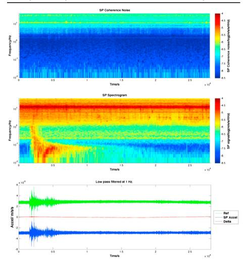
Fig. 16 Record teleseismic earthquake detected by QM SP1 in Oxford UK: spectrogram of the incoherent noise with respect to the reference sensor, signal spectrogram (middle) and time series (bottom, for a reference seismometer, green, for the SP in blue with the difference in red) for a  $M_w = 7.7$ , 29 km SW of Agriha, Northern Mariana Islands at 2016-07-29 21:18:24 UTC. The red time signal is the one used for the coherence noise spectrogram
