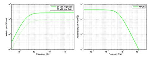
**Fig. 53** Solid lines: Generic shape of the Transfer functions of the SPs for the VEL output (left) and for the MPOS output (right). On the left, the dashed line is the low gain VEL output. The Full Scale Range of SEIS-AC is 25 Volt for SP VEL (with 24 bits) and 10 Volt for SP POS (with 12 bits for A/D and 16 bits after averaging)
