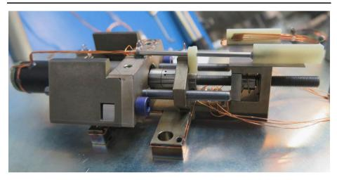
Fig. 44 Re-centering mechanism from the top and from the side. A lead screw is driven by a stepper motor through a 1:256 gear box and a flex coupling to displace the mechanism. Two parallel guides prevent the motor gear box to rotate. To minimize overall mass, the motor is on the moving part. The re-centering mechanism fits in a  $86 \times 36 \times 22$  mm<sup>3</sup> volume. The motor and gear box have a 10 mm diameter
