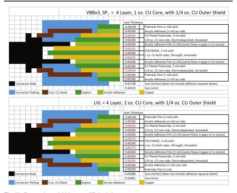
Fig. 66 Construction and thicknesses of Tether belts
