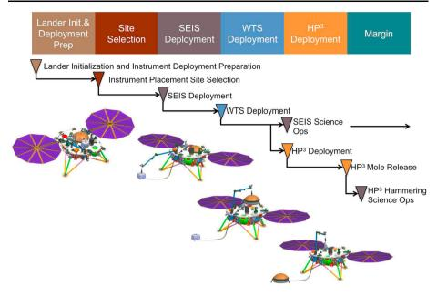
Fig. 26 Deployment process of the SEIS experiment following the landing and prior to the HP3. This does not detail the deployment internal to the SEIS sensor assembly after Sensor Assembly deployment on the ground
