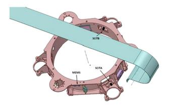
The number of sensors allows mapping the temperature of the instrument which is a key point for seismometer performance. The temperature sensors used to monitor the health of SEIS are digitized with a resolution of 12 bits while the sensors dedicated to science on VBBs and Levelling system feed respectively a 16 and 24 bit ADC for better resolution.
