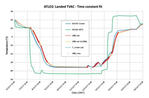
Fig. 110 Comparison data vs. temperature calculated with 1st order filter
