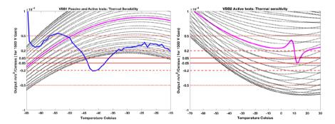
**Fig. 47** VBB 1 & 2 Thermal Sensitivity performances. VBB2 has higher thermal sensitivity at cold that exceed TCDM capabilities at low temperature. VBB2 meets its requirements over  $-55^{\circ}$ C. VBB1 is compliant over the full range. Color and lines definitions are the same as the right Fig. 46. Only the active tests results are shown for VBB2
