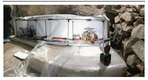
Fig. 80 Setup for SEIS QM test in the Black Forest Observatory mine seismic vault. EBOX on the left, sensor assembly with "cuvinette" on the right. Once the tent was closed the reference seismometers were installed on the pillar in the foreground
