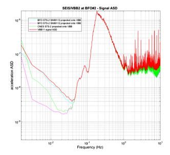
a controlled schedule context, but might also not be so surprising as a  $10^{-8}$  m/s<sup>2</sup>/Hz<sup>1/2</sup> noise level is equivalent to an instrument tilt of about 1.2 nano-radian/Hz<sup>1/2</sup> which might be easily induced by convection forcing on the instrument. Further analysis identified that the recorded VBB noise was likely related to the temperature noise induced by pressure transient variation in the small vacuum chamber (Fig. 93).
