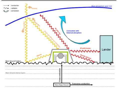
Fig. 105 Schematic of the SEIS sensor assembly environment
