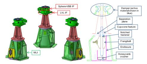
Fig. 74 Cradle Dampers (on left) and internal design of the cradles with the release mechanism (on right). The cradles are 185.5 mm height
