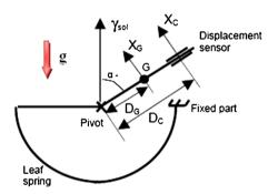
The configuration of the mechanical pendulum is such that the center of mass of the mobile part is above its axis of rotation. This configuration generates instability or a negative stiffness, which reduces the pendulum's balancing spring and pivot stiffness. The natural frequency of the pendulum can then be expressed as:
