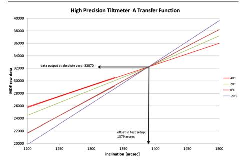
Fig. 102 Temperature calibration curves for HP tiltmeter, measured at  $-20^{\circ}$ C to  $40^{\circ}$ C in  $20^{\circ}$ C steps as described in the text
