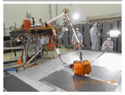
Fig. 12 The Sensor Assembly being deployed on the ground during DST#3 (Deployment System Test). Two segments of the tether (TSA-1, part of TSA-), the Tether Storage Box, Field Joint and part of the Load Shunt Assembly are also visible
