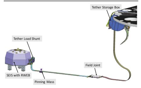
**Fig. 65** Tether System overview, Deployed Configuration. The TSA-3 and TSA-4 between the Tether Storage Box and the Ebox are unchanged from. The distance from the center of the Sensor Assembly of SEIS and the point below the Tether Storage Box is about 1.40 m in this configuration
