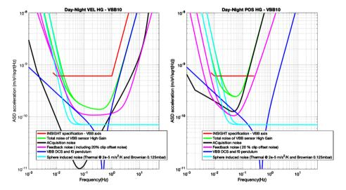
**Fig. 89** Noise model of one VBB axis in Mars conditions, for Night and Day conditions, for both the VEL (left) HG and POS (right) HG. For LG, the acquisition noise will be respectively 3.2 and 4.5 larger for VEL and POS output respectively
