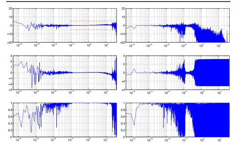
Fig. 94 The transfer function (TF) of SP determined from coherence testing shown in amplitude and phase. The requirement of  $\pm 5$  dB flatness within the bandwidth of SP is shown. The TF determination is valid within the bandwidth where the coherence is high, allowing extension of SP meeting the TF requirements to 0.006 Hz
