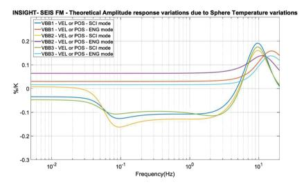
Fig. 87 SEIS VBBs Theoretical VBBs Amplitude Response variation wrt Sphere Temperature from feedback actuator thermal sensitivity measurements. At periods larger than  $100 \, \text{s}$ , the transfer function sensitivity is  $< 0.05\%/^{\circ}\text{C}$ , leading to 2.5% over the  $50^{\circ}\text{C}$  climatic variation between the coldest and hottest temperature of the VBBs over one Martian year
