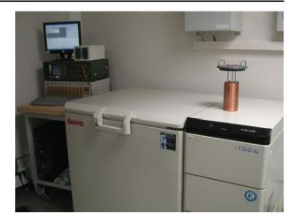
Fig. 98 Dry Heat chamber
