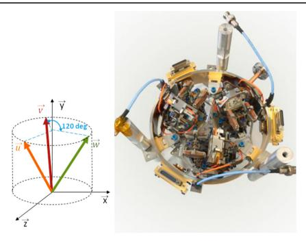
**Fig. 34** The 3 VBB sensors in the spherical evacuated container (right) which has an outside diameter of 198 mm. Their three sensing directions form the tetrahedron shown on the left
