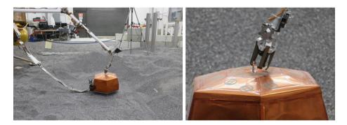
Fig. 29 SEIS Deployment (left) and grapple release (right)
