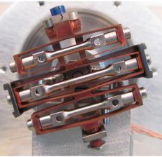
Fig. 45 Thermal Compensator Device Mechanism. Two thermal compensation devices are mounted on a shaft. A tuning mechanism allows tuning of their orientation in a vertical plane. It is composed of a stepper motor, a 1:256 gear box and a worm screw. The compensation device is 37 mm × 37.1 mm and can extend 12 μm per °C. The orientation mechanism is 43.2 mm long. Its motor and gear box are 8 mm in diameter
