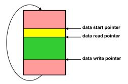
by the lander computer. The data start pointer is set to the page that contains the oldest data and the data write pointer is set to the first page where new data can be written. When a new packet is stored, it is stored where the data write pointer is set to and then this pointer is advanced. Data are deleted by advancing the data start pointer. If any of the pointers reaches the end of the area, then the pointer is moved to the start of the area when advanced.
