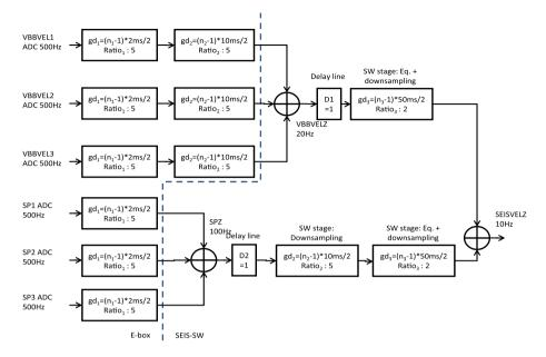
**Fig. 117** Example of SEISVELZ production chain by Ebox (on the left side of blue dashed line) and FSW (on the right side of blue dashed line) from SP and VBB channels. The final product (SEISVELZ at 10 sps) is provided in the continuous data flow
