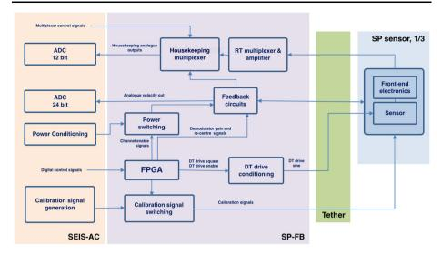
Fig. 52 A schematic of the SP electronics. SEIS-SC, the SEIS acquisition electronics are installed in the Ebox of the lander while the SP sensors are deployed on the Martian surface on the SEIS instrument assembly
