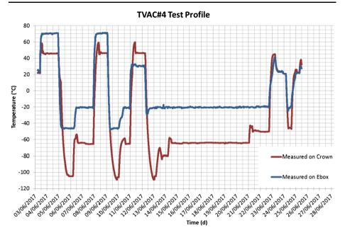
Fig. 109 TVAC#4 profile as realized
