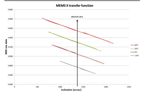
Fig. 103 Temperature calibration curves for MEMS tiltmeter, measured at  $-20^{\circ}$ C to  $40^{\circ}$ C in  $20^{\circ}$ C steps as described in the text
