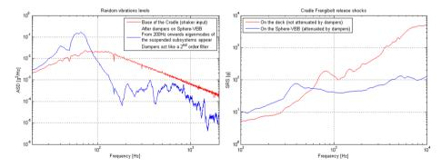
Fig. 75 Cradle damping efficiency. The left figure provides the damping of launch vibration, while the right figure provides the damping efficiency during cradle release. Red lines are those on the deck and blue lines are the acceleration levels at the SEIS assembly
