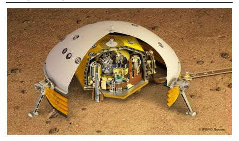
Fig. 22 Illustration of the RWEB and WTS configuration after deployment
