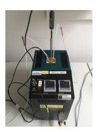
Since the flight model sensors could not be calibrated in the standard calibration baths, the calibration was performed in dry air with a very high constant time copper cylinder (see Fig. 97 and Fig. 98).
