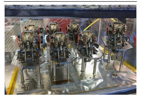
Fig. 38 All Flight and spare VBBs prior to the cherry-pick process which lead to the selection of the 3 Flight and the 3 spare units. Each VBB pendulum fits in a  $65 \times 100 \times 108 \text{ mm}^3$  volume
