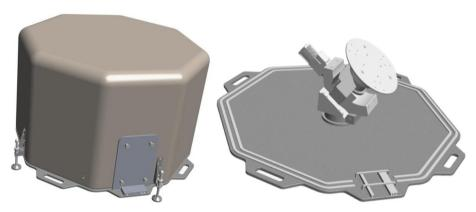
**Fig. 77** Left: Big thermal shield used for tests. Right: Aluminum plate and goniometer mounting. SEIS was mounted on the goniometer while the reference seismometers were installed on the plate or nearby
