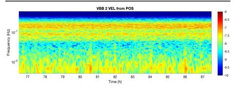
Fig. 93 Spectrogram of the VBB output in ground acceleration, during 10 hours of BFO tests with Earth configuration. The series of events seen at frequencies smaller than 0.01 Hz are likely related to pressure transient variations associated with the leak rate of the vacuum chamber used for the test and whose spectrum might be proportional to  $f^{-1}$ . The amplitudes shall be compared to those recorded by the STS-2s shown on Fig. 91
