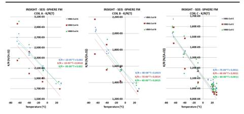
**Fig. 86** SEIS VBBs Magnetic actuators ratios of the force coefficient by the internal resistance with respect to Temperature. Coil A, B, C are the integrator, derivator and calibration coils respectively (see Sect. 5.1.5). Measurement errors remain large
