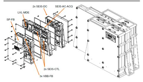
Fig. 20 The EBox and its electronic boards. The E-box is 243.8 mm in height. The top is  $303.5 \text{ mm} \times 125.5 \text{ mm}$  while the bottom is  $343.5 \text{ mm} \times 169.5 \text{ mm}$  due to mounting structures
