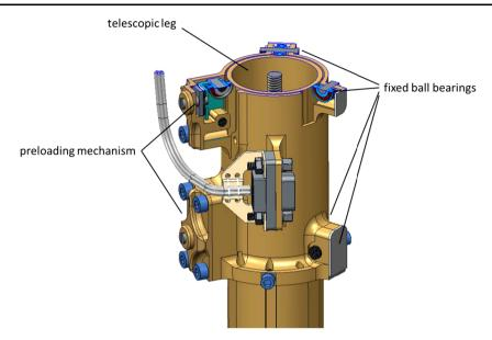
Fig. 54 Linear guidance of the telescopic leg. The diameter of the telescopic length is 25 mm
