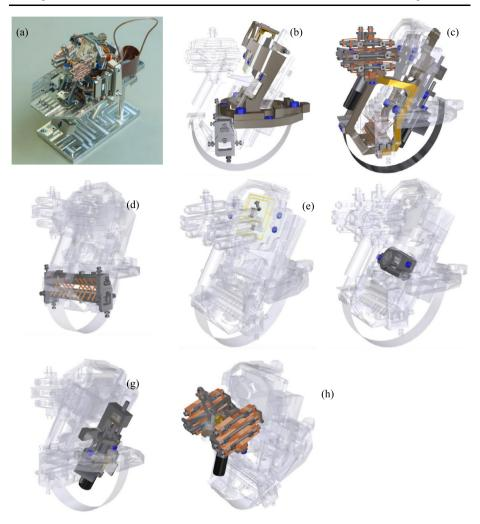
**Fig. 37** (a) One of the VBB sensor with Earth mass and VBB pendulum CAD views, illustrating the different functions of the sensor, (b) the fixed part, (c) the moving part, (d) the pivot, see Fig. 36, (e) the displacement Transducer, see Sect. 5.1.4, (f) the Feedback coils, see Sect. 5.1.5, (g) the re-centering motors, see Sect. 5.1.6 and Fig. 44, (h) the Thermal Compensation System, Sect. 5.1.8 and Fig. 45. A VBB pendulum fits in a  $65 \times 100 \times 108$  mm<sup>3</sup> volume
