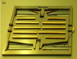
vertical suspension to attenuate the effect of temperature changes on the SP output (Liu and Pike 2015).
