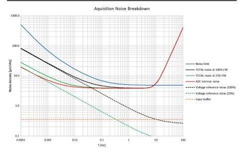
Fig. 64 The acquisition noise breakdown of VBB VEL channels (FSR =  $\pm 25$  V, 1 LSB = 3  $\mu$ V)
