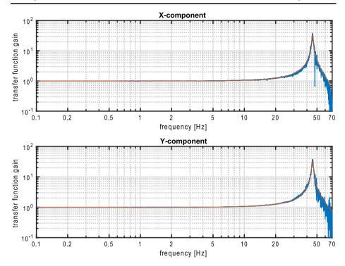
Fig. 104 Measured (blue) and modeled (red) gain of the horizontal transfer functions in the LVL baseline configuration (all legs extended by 0.5 mm). Masses, leg lengths and values of  $k_h^p$  of the model were set to those of the measurement, whereas parameters  $k_h^g$ ,  $C_h^g$  and Q were adjusted to fit the data
