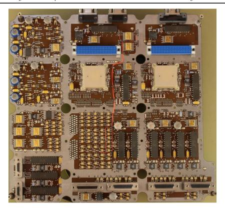
Fig. 58 The SEIS-AC acquisition electronics including redundancy
