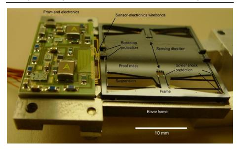
Fig. 49 The SP sensor mounted on its frame and connected to the proximity electronics
