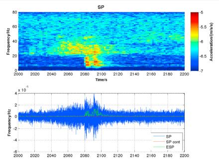
Fig. 15 Record of local earthquake detected by QM SP1 in Acton, California: spectrogram (top), time series (bottom) for a  $M_w = 1.4$  ENE of Colton, California, occurred on July, 17th, 2016, 06:34:11 UTC. The time series show the full 80 Hz bandwidth from 200 sps (labeled SP), downsampled to the continuous stream of 2 sps (cont. SP) and using the energy in a 4 to 16 Hz filter downsampled to 2 sps (ESP)
