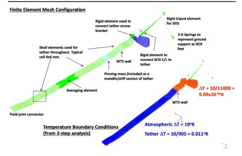
Fig. 67 Finite element mesh configuration for thermal and elastic models of the tether
