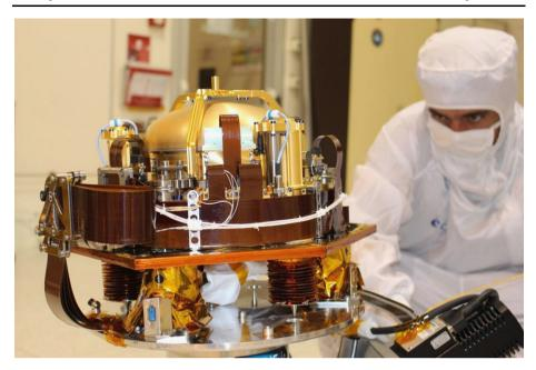
Fig. 11 SEIS Sensor Assembly (SA) without the RWEB
