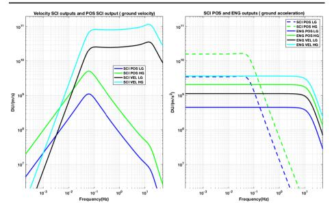
Fig. 42 FB transfer function at  $-55^{\circ}$ C for unit VBB10. On left are the Transfer functions for the ground velocity and at right are those for the ground acceleration, in Digital Unit (DU) per ground velocity (m/s) or ground acceleration (m/s<sup>2</sup>)
