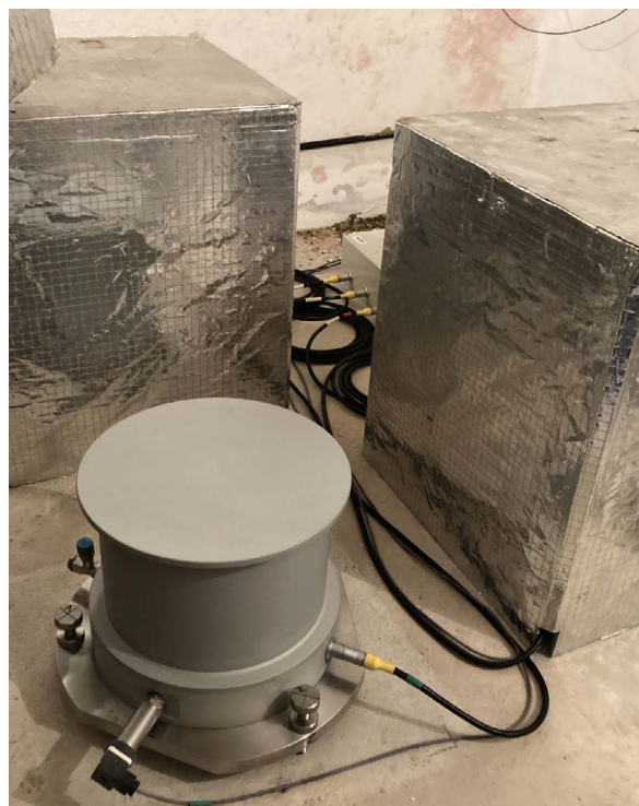
Work on two stations equipped with STS-1 sensors. Left, UNM station (Mexico, June 2024), right, SPB station (Brazil, October 2024). On the right, the cover of one of the three STS1 sensors has been removed, making the sensor visible.
