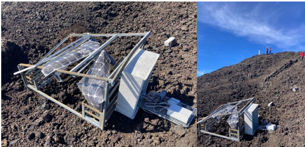
Figure A1: DERG station (Dolomieu est) washed away and destroyed by cyclone Belal (photo January 18, 2024).
