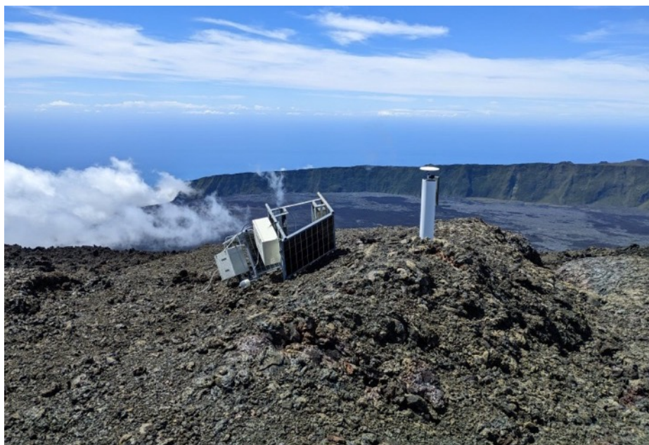
Figure A2: DSRG station (Dolomieu sud) washed away and destroyed by cyclone Belal (photo January 18, 2024).
