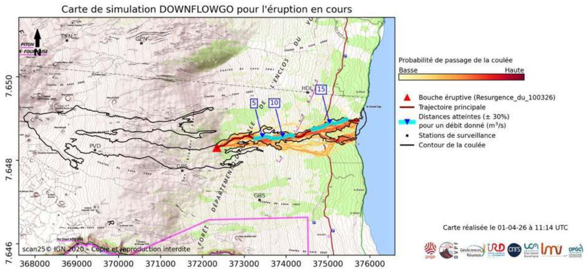
Figure 18: Numerical simulations of probable lava flow inundation paths based on the main resurgence point as of March 10, 2026, on the main southern branch. See the legend in Figure 17 for further details (©OPGC-LMV-OVPF-IPGP).
