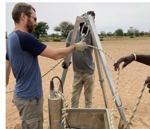
Improving seismological signals at SOK (Senegal). Aerial view of the site when the well was drilled in 2022 (left) and reinstallation of the T360 sensor in the 20 m well in July 2023 (right).
