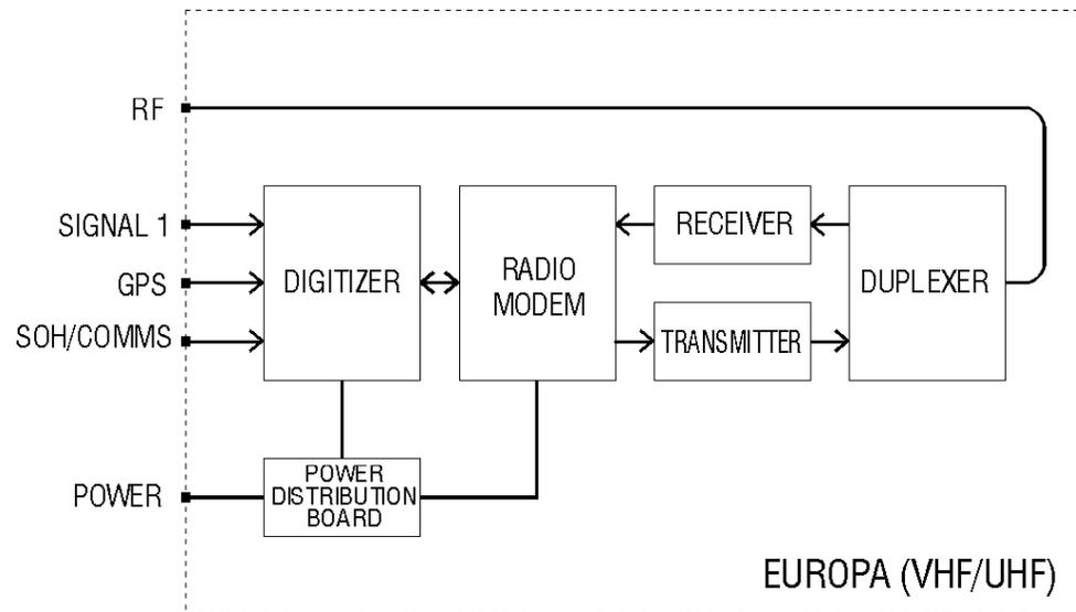
**Figure 2: Europa (VHF/UHF) block diagram**
