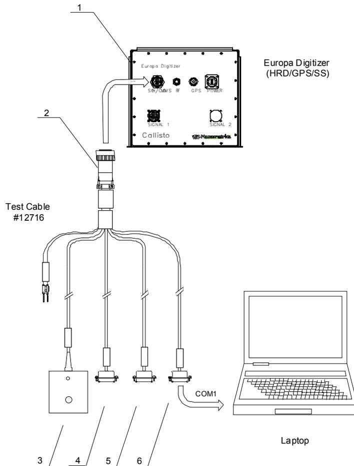
**Figure 6: Europa (HRD/GPS/SS) test/configuration cable**
