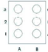
**Figure 12: Pinout for J12, J3, J4, J5, J6**
