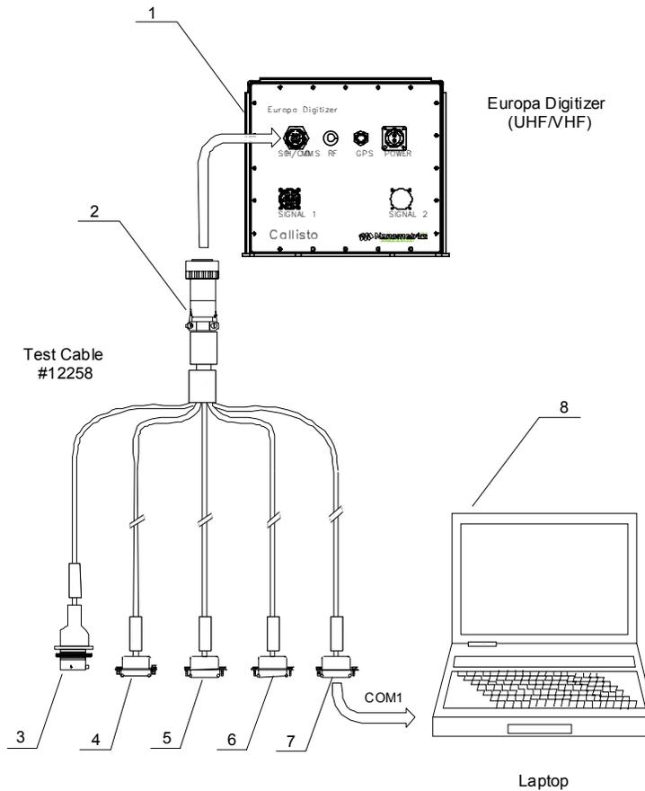
**Figure 4: Europa (VHF/UHF) test/configuration cable**
