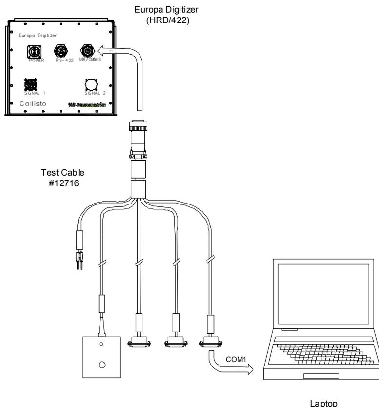
**Figure 9: Europa (HRD/422) test/configuration cable**
