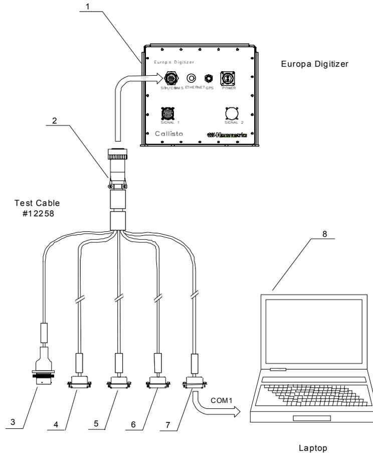
**Figure 10: Europa HRD test/configuration cable**
