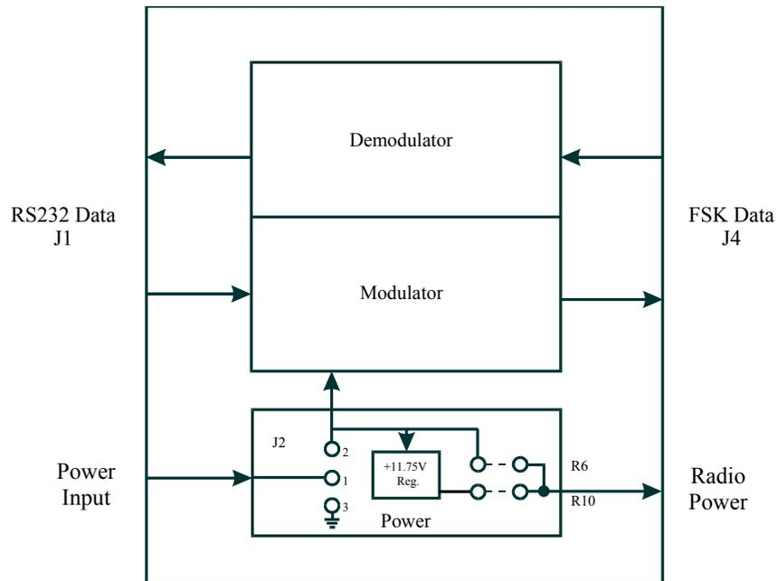
*Figure 3: Block diagram of the radio modem*
