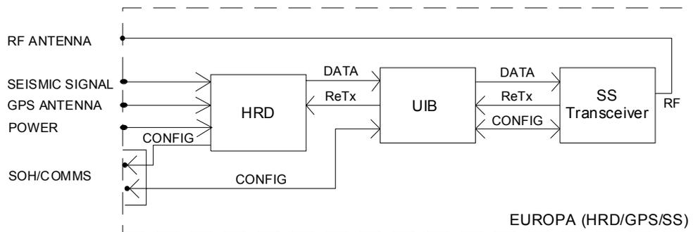
*Figure 5: Europa (HRD/GPS/SS) block schematic*
