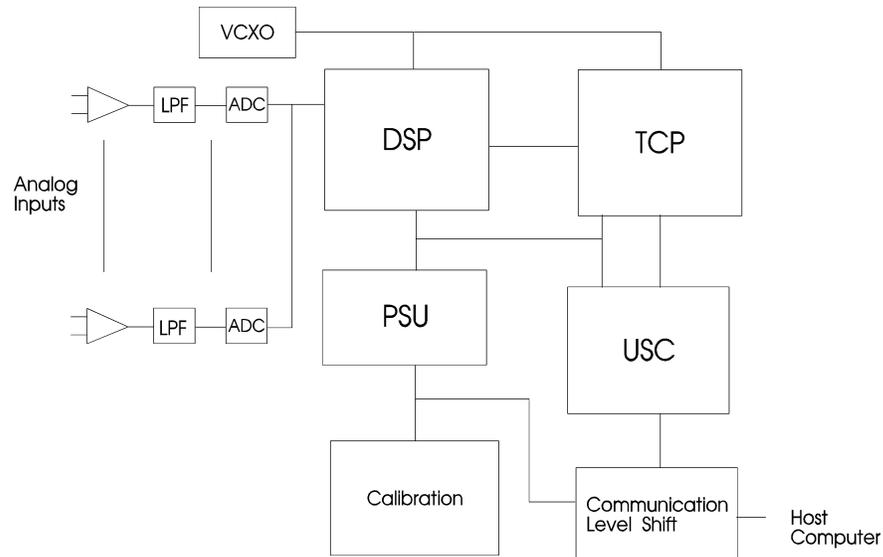
*Figure 1: Block diagram of the digitizer module.*
