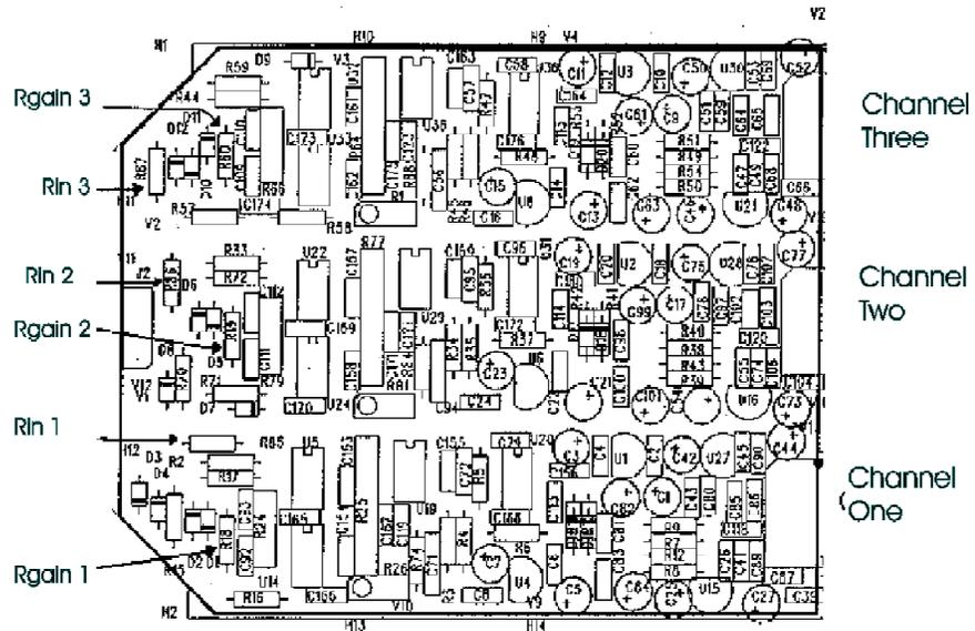
Figure 11: Gain and damping resistors on the ADC card
