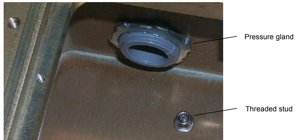
Figure 2: Location of threaded stud for securing the central strength member
