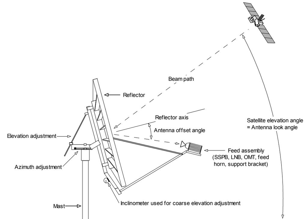
**Figure 10-4** Antenna azimuth
