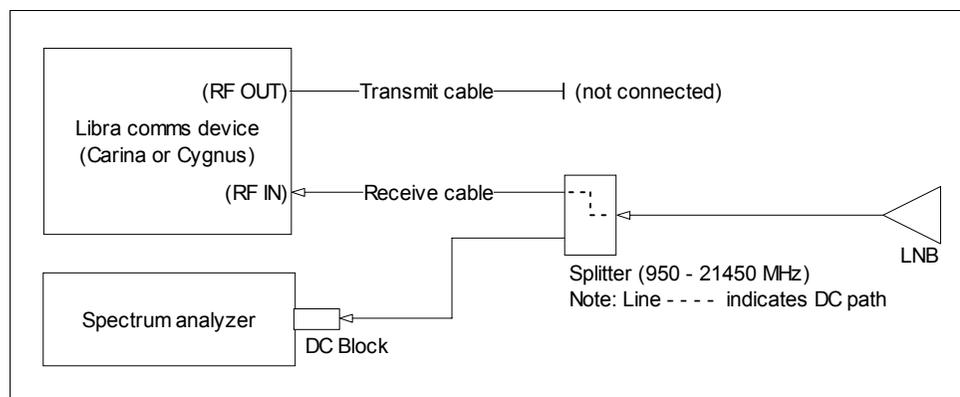
3. Power up the spectrum analyzer and set the configuration (for example, as shown in Figure 12-7).
