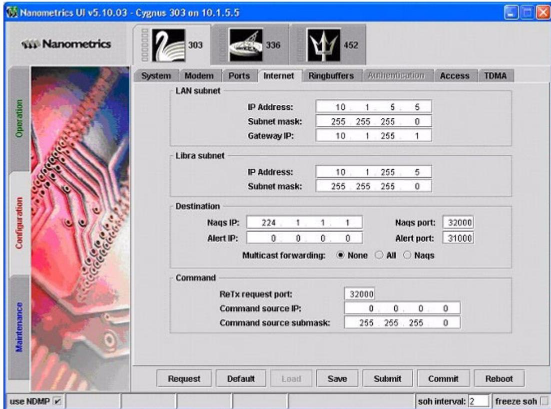
Figure C-12 shows an example IP configuration for a Libra network. You can also set up one large subnet to include every Cygnus if you wish.
