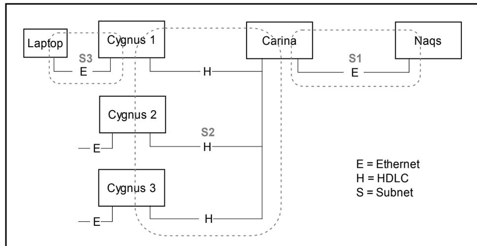
Each remote Cygnus transceiver and each central site Carina VSAT modem has two network interfaces:
