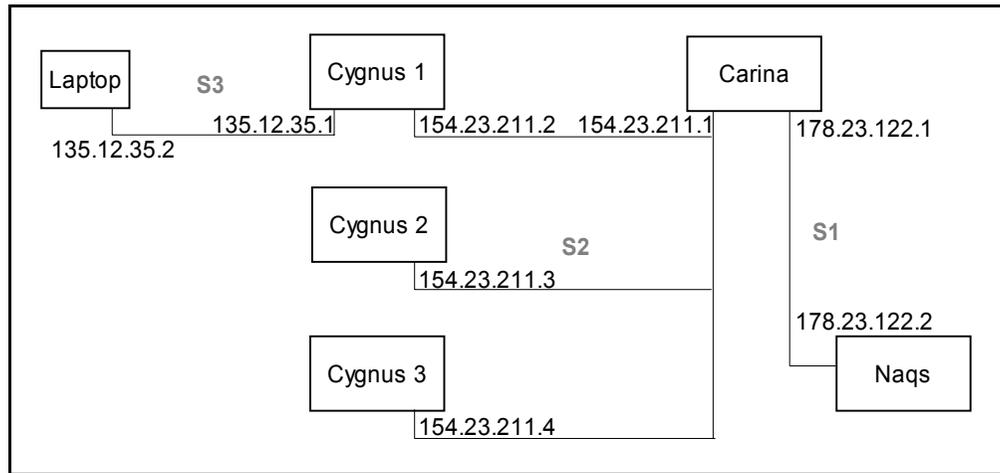
The Naqs computer is set to IP address 178.23.122.2, subnet mask 255.255.255.0 (that is, width of 24), and gateway 178.23.122.1. If the network is connected to the Internet, the gateway to the Internet should be added to the routing table for the acquisition computer.
