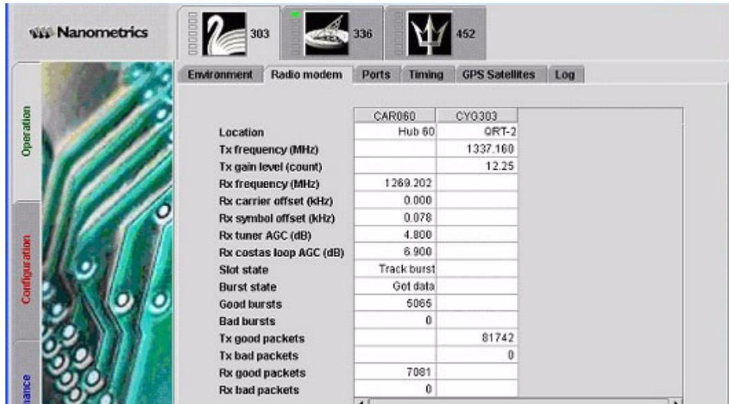
3. Carina transmits one TDMA authorization packet in every burst. Check for this activity on the Carina Operation > Radio Modem screen:
