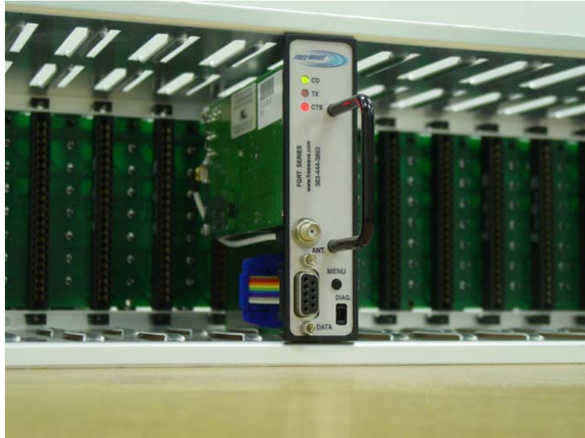
Figure 2. T-Series Installed In Loop Detector Rack
