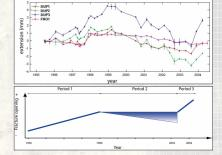
Extensometer monitoring network. It has been set up on La Soufrière in 1995 [*David*, 1998] and consists presently in 17 stations on the main fractures of the lava dome. Measurements take a full day in the field with two rators and are repeated every 3 months
