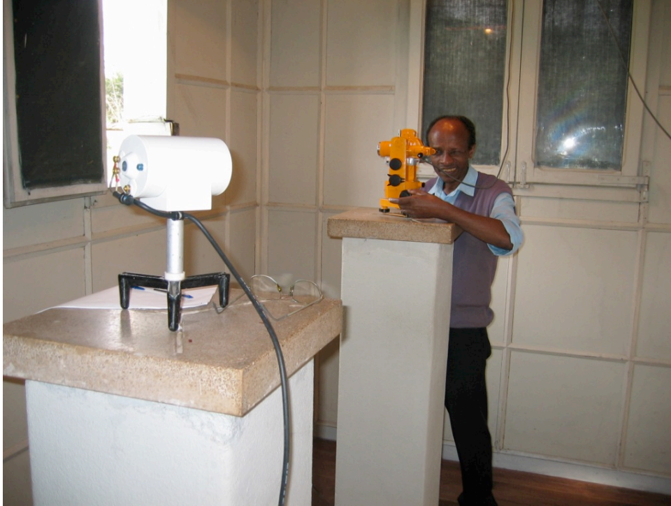
Figure 3: Absolute measurement using a “DI-flux” and a scalar magnetometer at Addis Ababa magnetic observatory. (The photographed observer is Abebe Albie Toro.)
