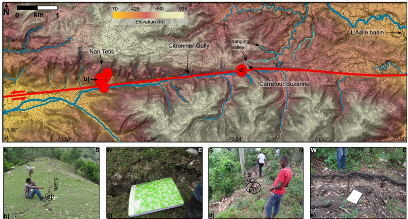
Figure 6. (a) Fault mapping and coseismic cracks in western L'Asile. LiDAR topographic contours are 5-m intervals. Note the locations of the photographs in (b, d). (b) Crack in Nan Tetis. The land dips to the south. (c) Zoom showing apparent vertical offset in (b). The green and white object is a notebook for scale. (d) Crack in Carrefour Suzanne. The land dips to the south. (e) Apparent vertical offset of the Carrefour Suzanne crack.
