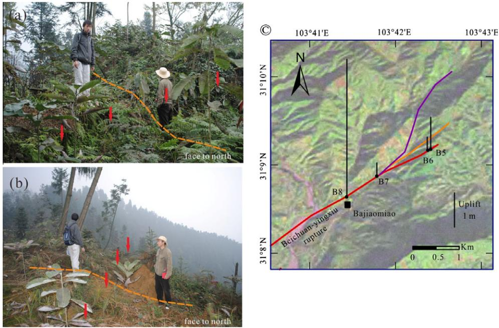
**Fig. 3.** (a) Rupture photos at point B5; (b) Rupture photos at point B6; and (c) the map of the Beichuan-Yingxiu rupture shown as the red line in the Bajiaomiao area. The yellow line is the boundary between the Peng-Guan massif and sedimentary rocks, and the purple line is the conjectured rupture in reference. The yellow dashed lines represent the topography lines of fault scarps.
