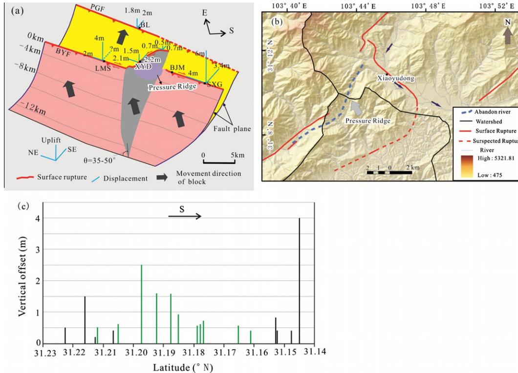
**Fig. 9.** (a) Mechanism model for the Xiaoyudong fault rupture (the fault planes are after Hubbard et al., 2010). (b) Geomorphologic features in the Xiaoyudong area. (c) Vertical offset of the Xiaoyudong rupture and the Beichuan-Yingxiu rupture in the Xiaoyudong area along latitude.
