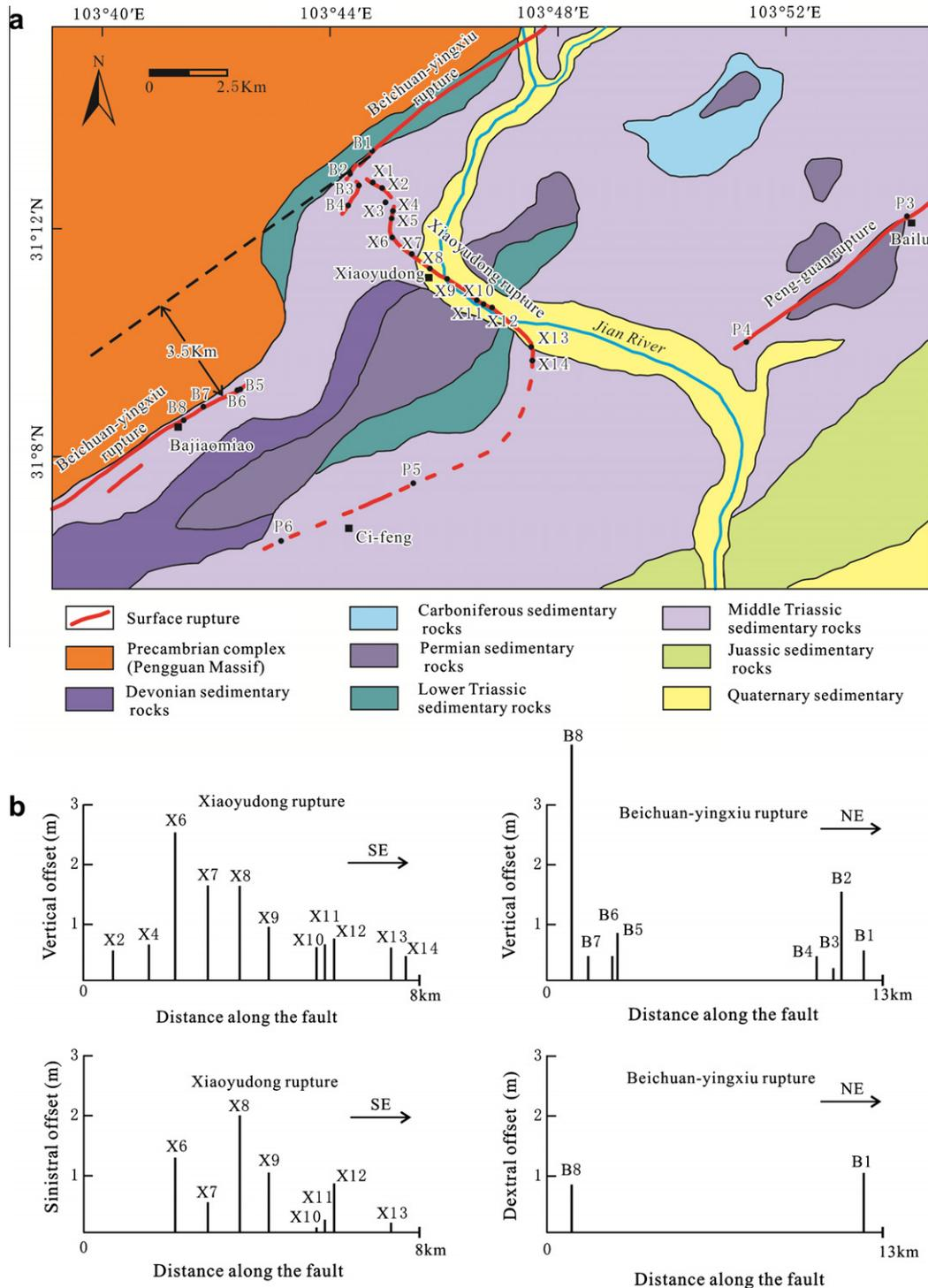
Fig. 2. (a) Distribution of the surface ruptures and geological map and (b) vertical and sinistral offset of the Xiaoyudong rupture and the Beichuan-Yingxiu rupture in the Xiaoyudong area.
