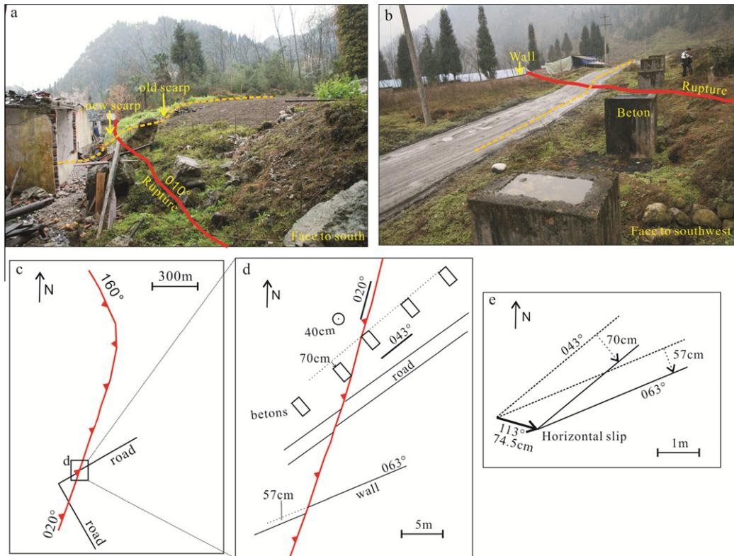
**Fig. 4.** (a) Rupture photo at point B2; (b) Rupture photo at point B4; (c) and (d) are the sketch maps of the rupture near B4 in a different scale; and (e) the horizontal slip of the rupture at B4. The yellow dashed lines represent the topography lines of fault scarps.
