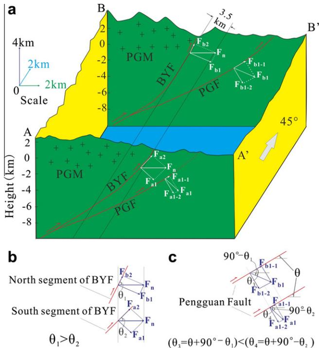
**Fig. 10.** Model explanation for two parallel faults being ruptured simultaneously (the position of profile A-A' and B-B' shown in the Fig. 8-b).
