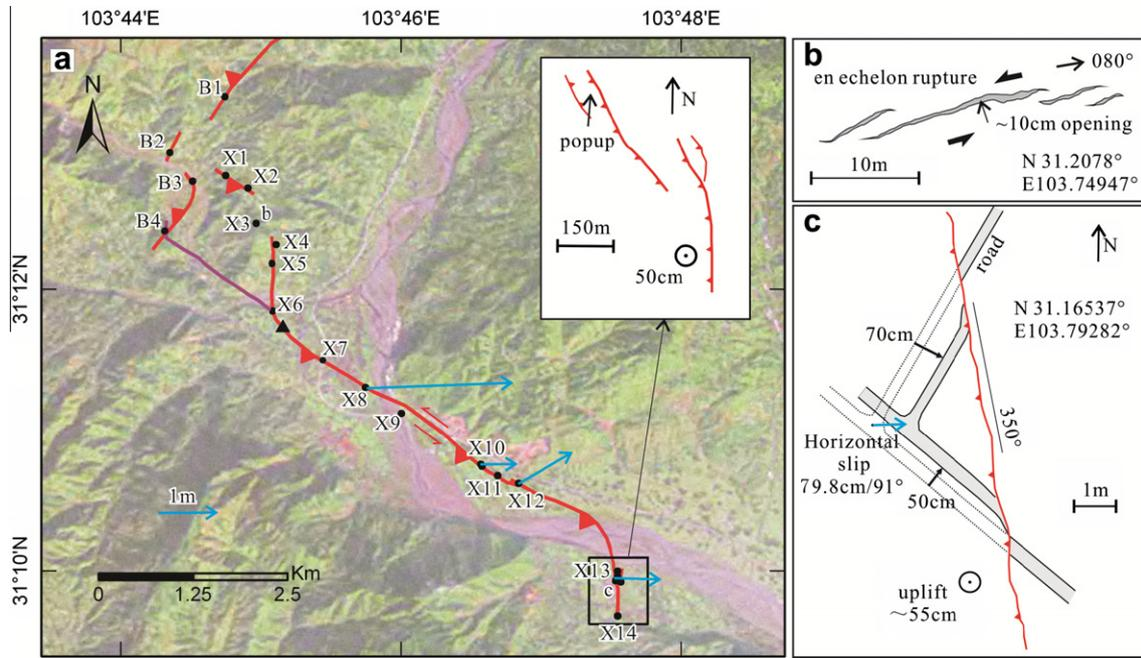
**Fig. 6.** Distribution of the Xiaoyudong fault rupture: (a) Locations of the investigation points (listed in the Table 2) and the co-seismic horizontal slip vectors (blue arrows); the purple line is the rupture at the northwest extreme of the Xiaoyudong fault suggested by Li et al. (2009) and Liu-Zeng et al. (2010). The black triangle is the location of the trench by Ran et al. (2010). (b) Sketch map of point X3; and (c) Sketch map and measured data of point X13 in detail.
