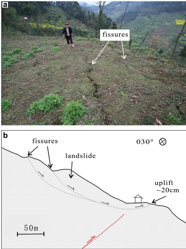
Fig. 7. Photo (a) and sketch map (b) of the fissures induced by sliding in the south segment of Peng-Guan fault. (The photo was taken at point P5 shown in Fig. 2).
