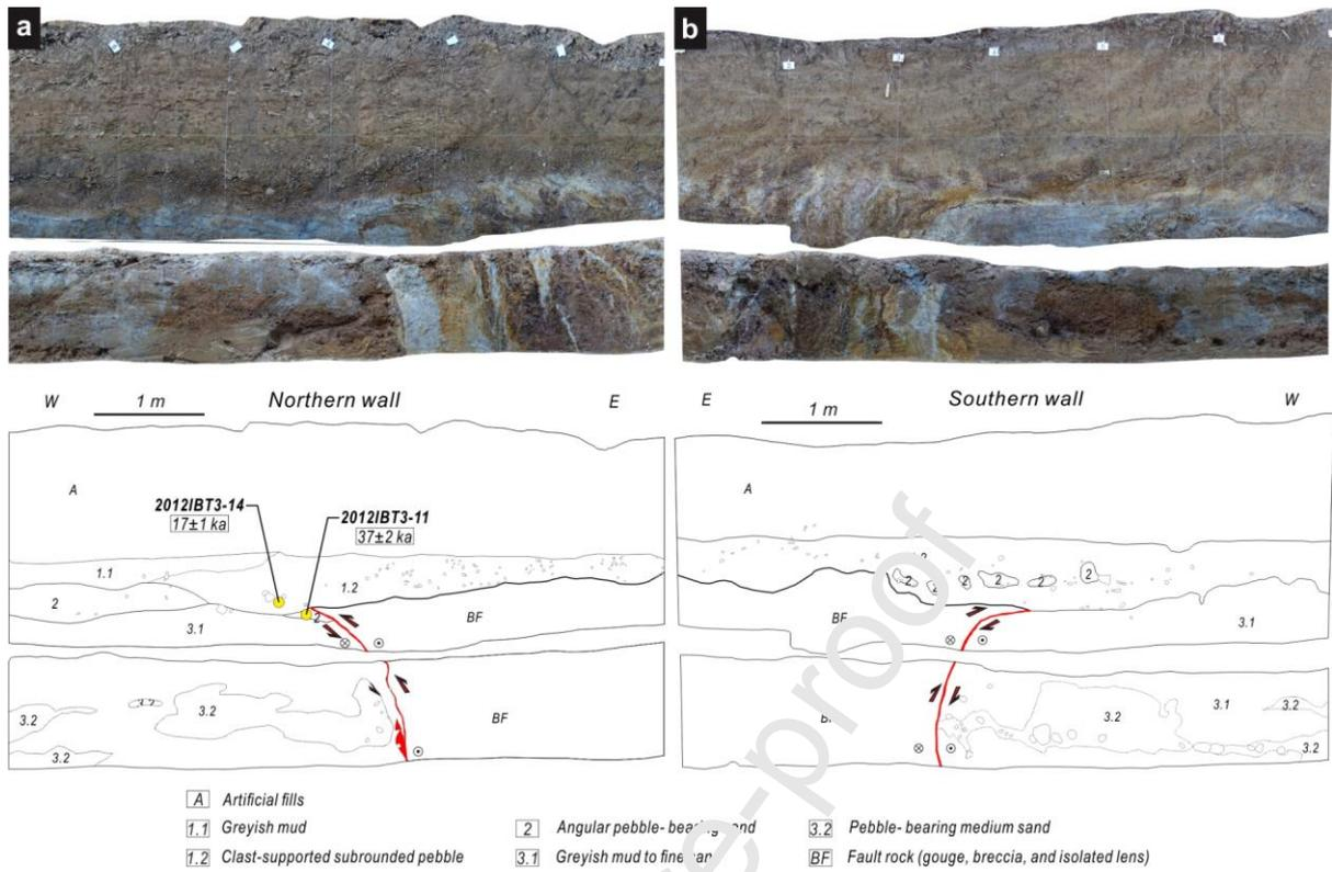
Fig. 8. Photographs and detailed sketches of the northern (a) and southern (b) walls of the IBN trench. The grid interval is 1 m × 1 m. Yellow circles indicate OSL sampling points with ages.
