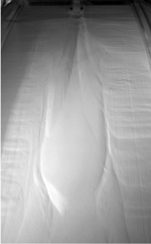
Figure 1. Typical channel and frontal lobe obtained with our experimental setup. The current inlet is visible at the top.
