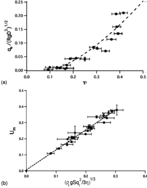
Figure 4. (a) Dimensionless sediment transport rate  $q_s / (R g D^3)^{1/2}$  versus shields number. (b) Average flow velocity  $U$  as a function of  $(\rho_f g S q_i^2 / 3 \eta)^{1/3}$ .
