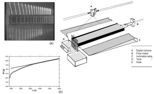
Figure 1. Schematics of the experimental setup. (a) Measurements of bed elevation by mean of a set of laser sheets projected on the river. (b) Cumulated sediment mass as a function of time at the flume outlet: about ten minutes after initiation of the flow, sediment discharge reaches a stationary state.
