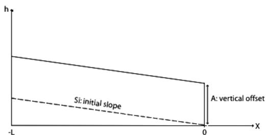
Figure 3. Representation of initial river bed which undergoes a vertical offset of magnitude  $A$ .  $h$  represents the bed elevation,  $x$  is the position along the bed river and  $L$  is the length of the flume.
