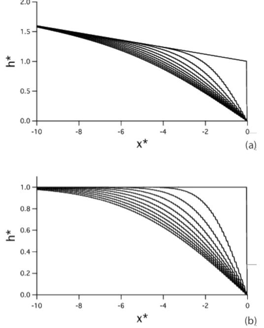
Figure 5. Dimensionless bed elevation  $h^*(x^*, t^*)$  from  $t^* = 0$  to 10. The dimensionless time step between two successive profiles is  $\Delta t^* = 1$ . (a)  $S_i = 0.03$  and  $S_C = 0.001$  (b)  $S_i = 0.0001$  and  $S_C = 0.0001$ .
