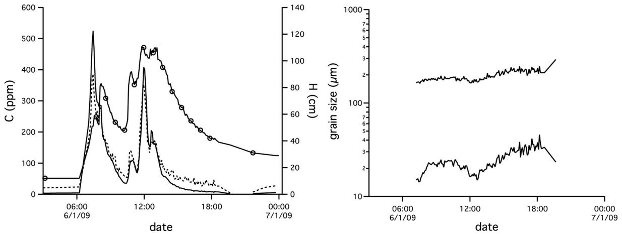
FIGURE 3: Data acquired during a flash flood on January 6th 2009. (a) Water flow depth (line with circles), volumetric concentration of suspended silt (solid line) and sand (dotted line) as a function of time ; (b) Average grain size of silt and sand particles as a function of time.
