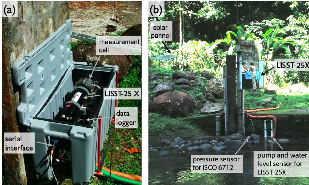
FIGURE 2: (a) Picture of the field adapted instrument showing the LISST-25 X and the measurement cell. (b) Image of the field test site on the Capesterre river. The sensor and the data logger are located at about 8 meters away from and 2 meter above (at low flow) the river bed while the pump is submersed into the stream.
