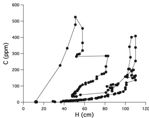
FIGURE 4: Plot of silt concentration versus water level for the same event as on Figure 3.
