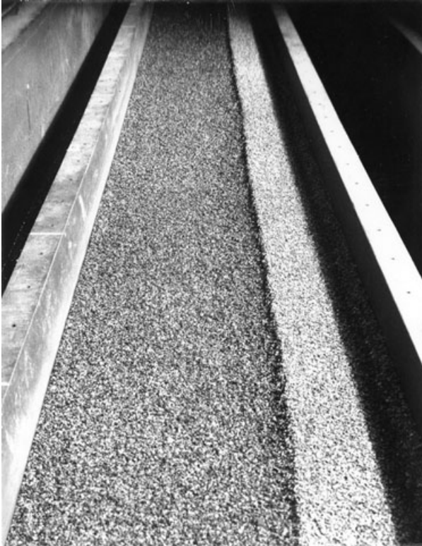
Fig. 2. Image of a stable self-formed mobile-bed channel in fine gravel. The width of the channel is about 29 cm. The flow, which was from bottom to top, has been turned off. The image is courtesy of P. Diplas.
