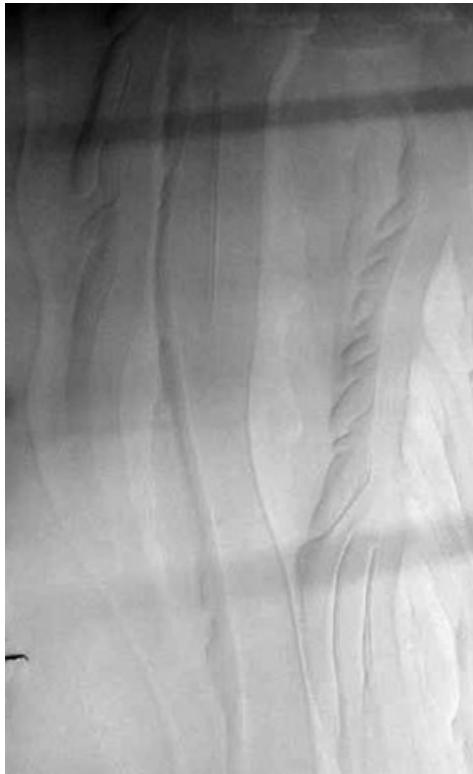
Fig. 11. View of levéed channels emplaced by a laminar or near-laminar turbidity current in the laboratory. Flow is from top to bottom. The width of the experimental flume is 2.15 m.
