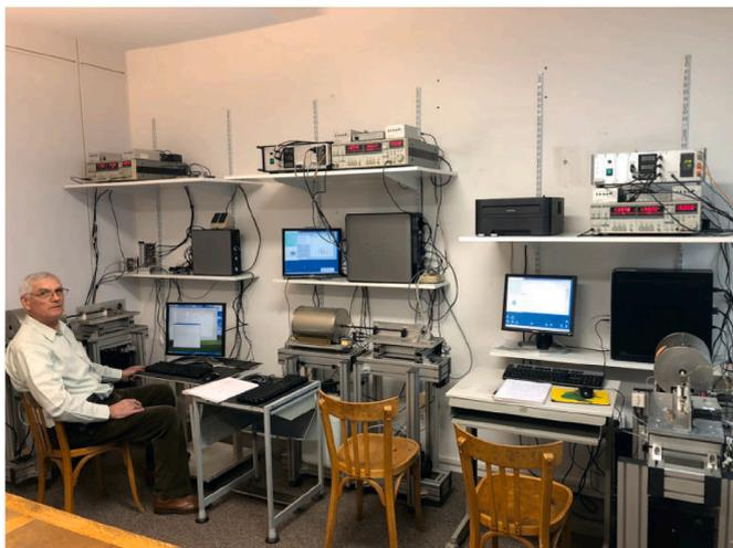
Fig. 1. Photo of the three Triaxe magnetometers available at IPGP and LAMS. Their builder, Maxime Le Goff, stands in front of them. @Yves Gallet.
