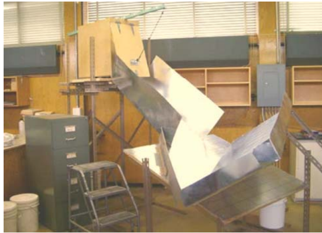
Figure 5.30. Photograph of laboratory apparatus used for deflected runoff experiments (Image courtesy of S. McDougall, University of British Columbia).
