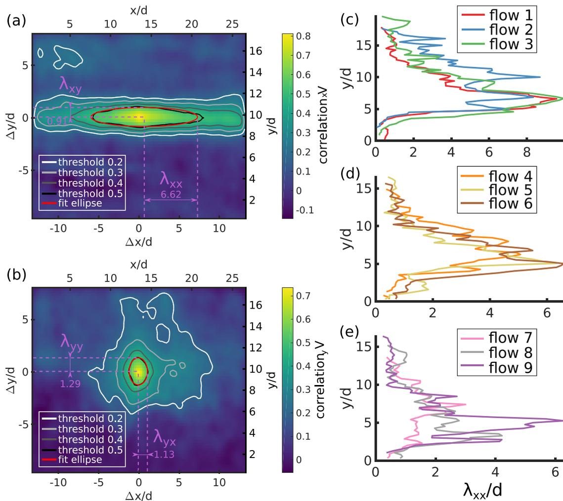
**Figure C2.** Example of spatial correlations between the (a) downslope and (b) base-normal components of fluctuating grain velocities, between the static point of coordinates  $(x/d = 14, y/d = 10)$  and all the others positions for the flow 2. Panels (c) to (e) correspond to the correlation length  $\lambda_{xx}$  of the horizontal velocity in  $x$  direction for all the flows.
