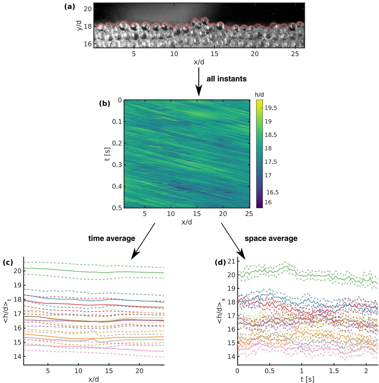
**Figure A1.** Heights of the flows: (a) example of flow interface detection (red line), (b) space and time height, thereafter averaged over (c) time or (d) space. Each color of panels (c) and (d) corresponds to a specific flow (see e.g., Figure 11 for detailed legend), while continuous lines correspond to mean values and dashed lines to one standard deviation either side of these means.
