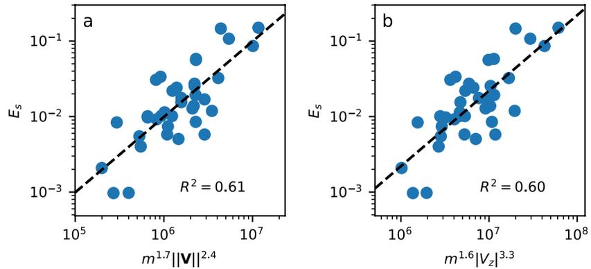
**Figure 12.** (a) Energy  $E_s$  of the seismic signal generated at each individual block impact, as a function of  $m^\alpha \|\mathbf{V}\|^\beta$ , for block mass  $m$  and modulus of the velocity before impact  $\|\mathbf{V}\|$ , with the exponents  $\alpha$  and  $\beta$  inferred to get the best fit by linear regression and (b) as (a), except with  $|V_z|$  rather than  $\|\mathbf{V}\|$ . All quantities are in SI units and rockfall data are from Hibert, Malet, et al. (2017).
