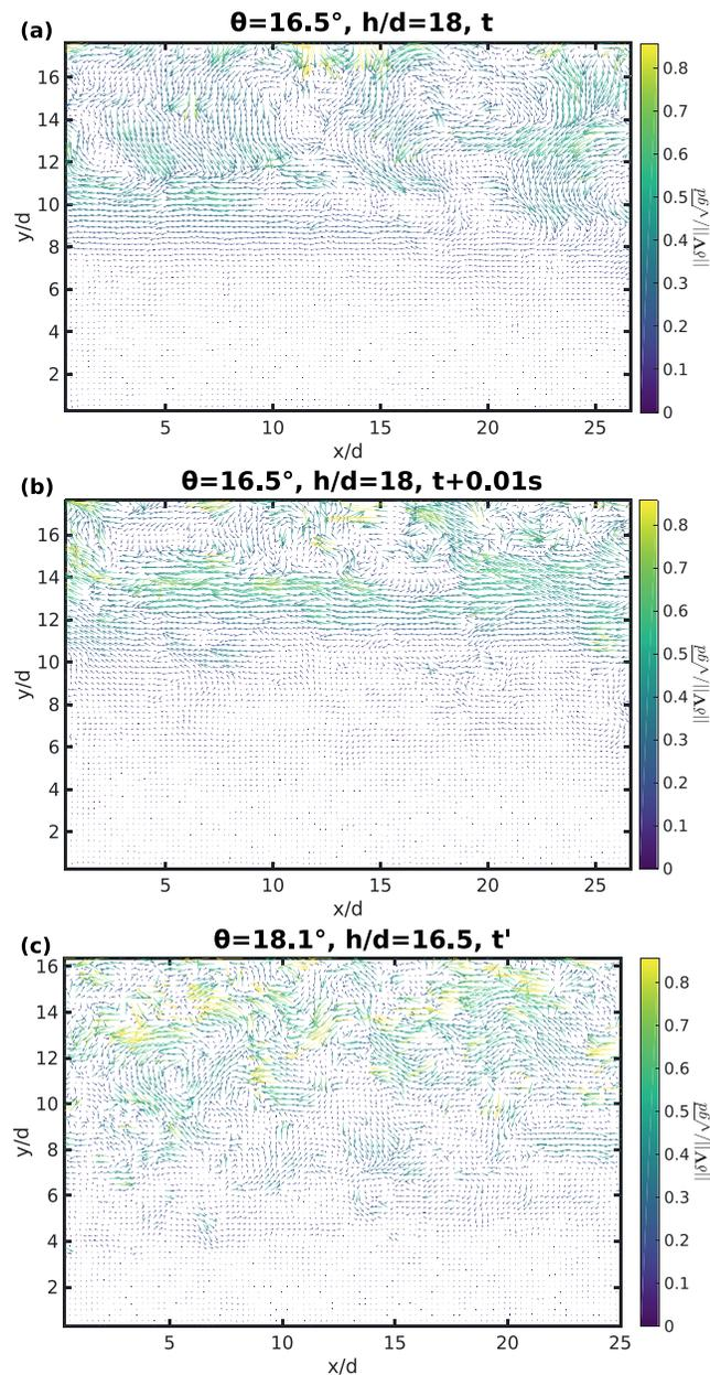
**Figure C1.** Map of velocity fluctuations obtained with Correlation Image Velocimetry for flow number 2 (a and b) and 9 (c) at instants  $t$ ,  $t + 0.01$  s, and  $t'$ , respectively ( $t$  and  $t'$  are arbitrary).
