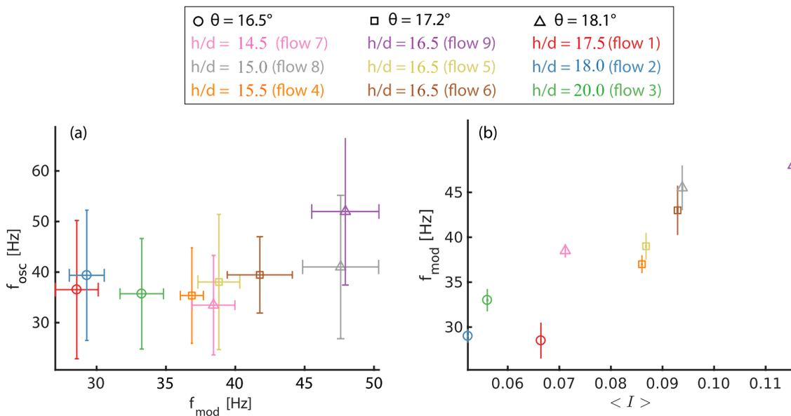
**Figure 10.** (a) Particles' vertical oscillation frequency  $f_{osc}$ , as a function of the frequency  $f_{mod}$  of the acoustic amplitude modulation. (b) Acoustic modulation frequency  $f_{mod}$  as a function of the average inertial number  $\langle I \rangle$ .
