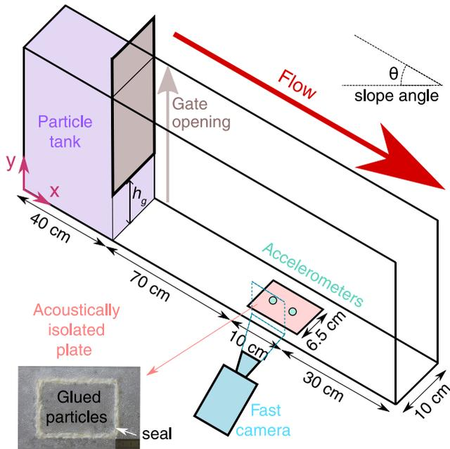
**Figure 2.** Setup, composed of a narrow inclined channel in which granular flows are created by opening the gate of the upstream tank that contains glass particles. The same particles are glued to the bottom plate to obtain a rough surface. The flow properties are measured using a high-speed camera and the generated acoustic waves by accelerometers fixed on the channel bottom.
