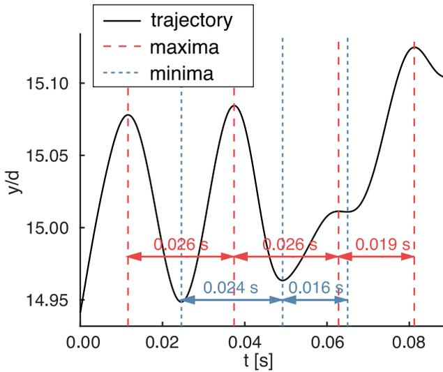
**Figure 4.** Example (from experiment 2) of vertical particle oscillations captured by Particle Tracking Velocimetry, for a particle located close to the surface of the flow: The smoothed trajectory demonstrates the calculation of the average period of the oscillations  $\tau \approx 0.02$  s.
