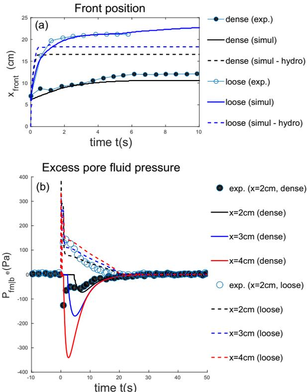
**Figure 3.** Time evolution of (a) the front position for both initial packing from experiments (dense  $\bullet$ - and loose  $\circ$ -) and simulations (non hydrostatic [dense  $-$ , loose  $-$ ] and hydrostatic [dense  $--$ , loose  $--$ ] pressures) and (b) the pore pressure below the column from experiments (dense  $\bullet$  and loose  $\circ$ ) at  $x = 2$  cm and simulations at  $x = 2$  cm (black),  $x = 3$  cm (blue),  $x = 4$  cm (red).
