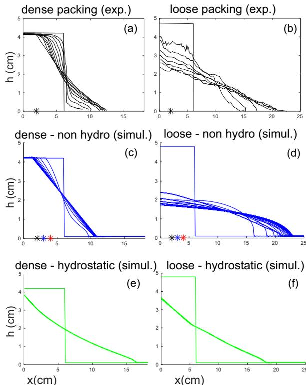
**Figure 2.** Granular mass profiles from experiments [top] and simulations (non hydrostatic [middle] and hydrostatic [bottom] pressures). Left: dense initial packing ( $\varphi_i = 0.6$ ,  $L_i = 6$  cm,  $H_i = 4.2$  cm) every 3s. Right: loose initial packing ( $\varphi_i = 0.55$ ,  $L_i = 6$  cm,  $H_i = 4.8$  cm) every 0.66s. The marker \* is the position where the time series of the excess pore fluid pressure is measured in experiments.
