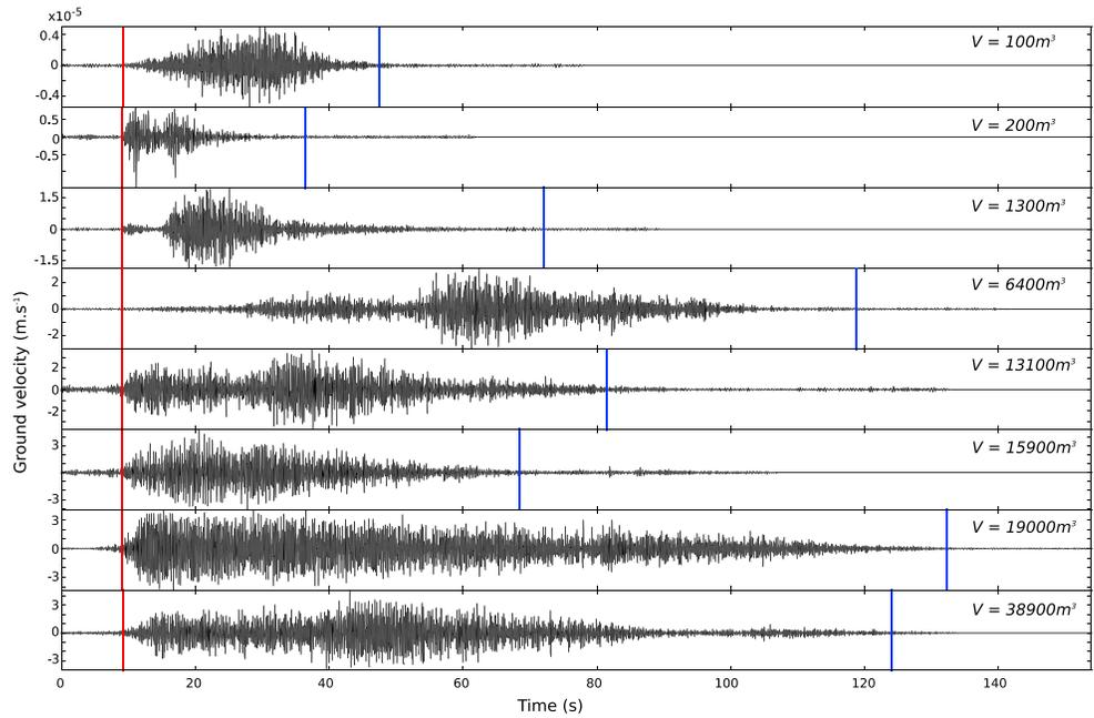
**Figure 2.** Examples of seismic signals generated by rockfalls of different volumes. The red and blue vertical bars show the beginning and end of the rockfall signals, respectively, detected using the method proposed by Hibert et al. (2014). These signals were all recorded at DSO station.
