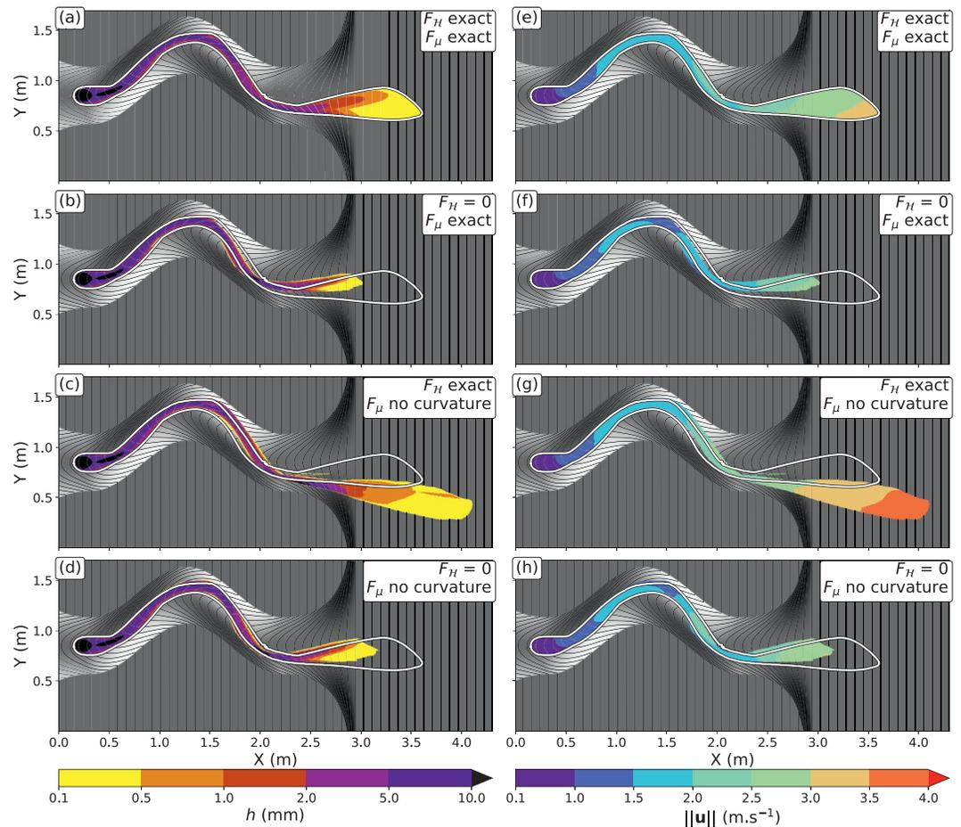
**Figure 7.** Same as Figure 6, but with the Coulomb rheology,  $\mu = \tan(15^\circ)$  and a slope  $\theta = 25^\circ$ . The contour interval is 4 cm. Simulation duration is 2.3 s. The kinetic energies are given in Figure 8.
