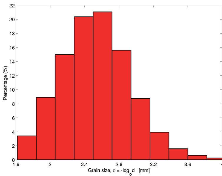
**Figure 1: Grain size distribution in the Tengger desert.** The sand bed exhibits a mean grain size of 2.39 ( $d=190 \mu\text{m}$ ).
