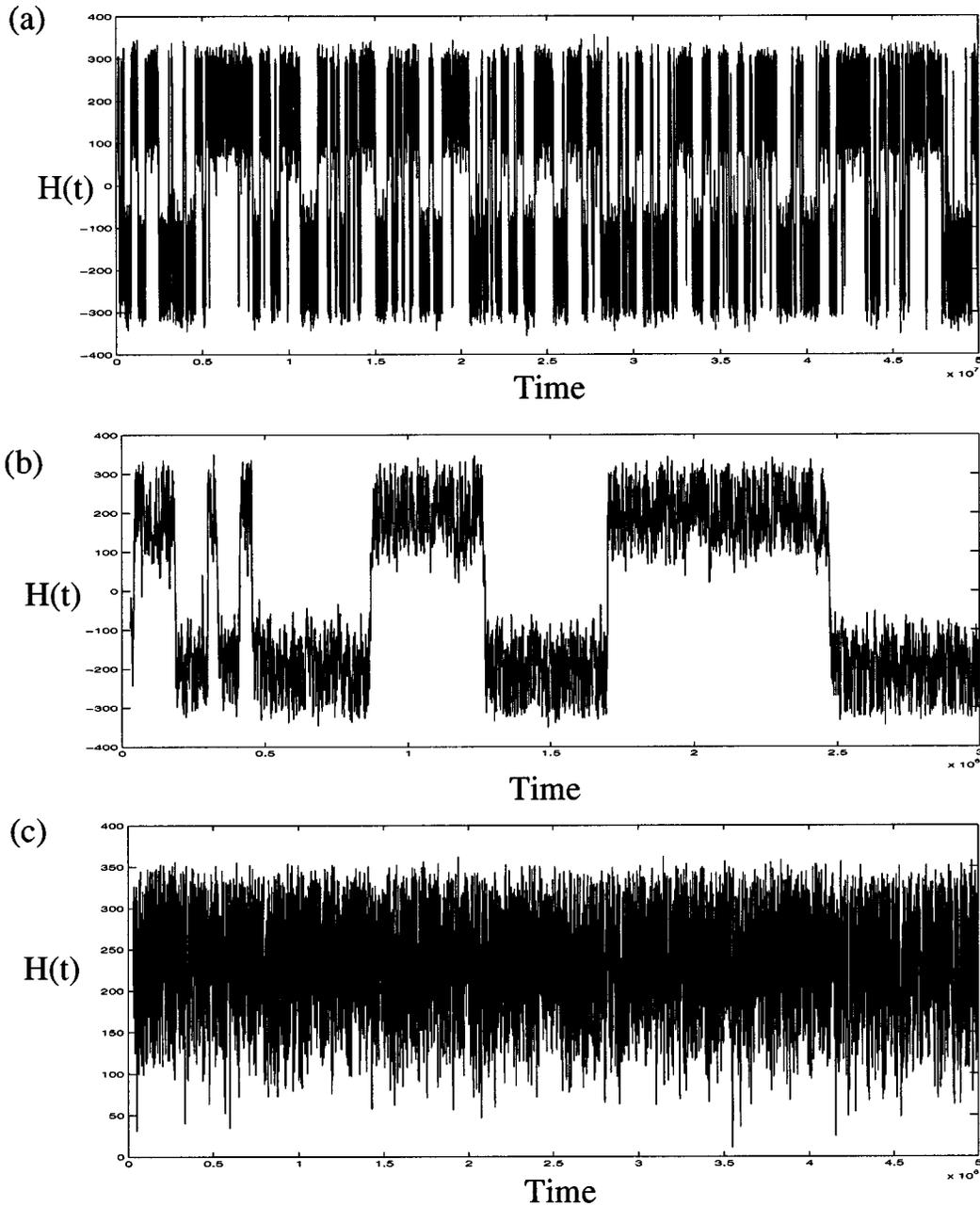
FIG. 12. Temporal evolution of the generated magnetic field intensity for a two-side cascade effect. (b) is a zoom of the first part of (a). Parameters of cascades: (a), (b)  $F_0=0.5$ ,  $\alpha_0=0.1$ ,  $\gamma_0=0.01$ ; (c)  $F_0=0.3$ ,  $\alpha_0=0.2$ ,  $\gamma_0=0.01$ . See other parameters of the modeling in Table I.
