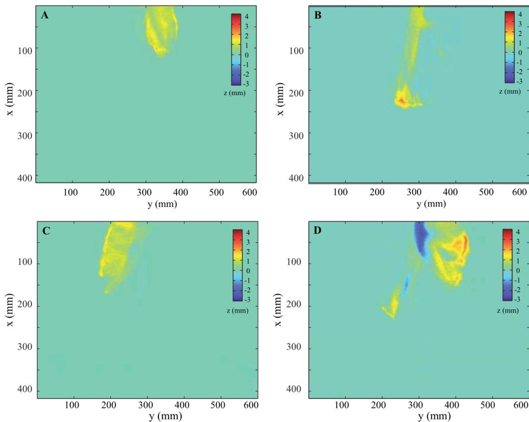
Figure 2 Example of a 2 minutes-long erosion/deposition sequence observed during an experiment. (A, B, C and D) Successive mass balances across the fan. These mass balances are calculated every 30 seconds from the fan topographic evolution. In green, yellow and red: locations with sediment deposition. In blue: locations with sediment erosion. Note the lobate shape of the successive deposits.
