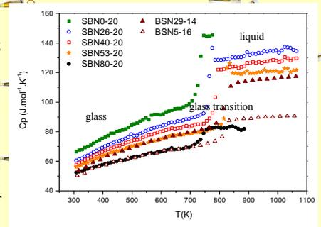
Heat capacities of the borosilicate melts. Measurements were made at IPGP between 300 and 1073K with a differential scanning calorimeter (DSC). △ and ▲ correspond to data from Y. Linard [1].
