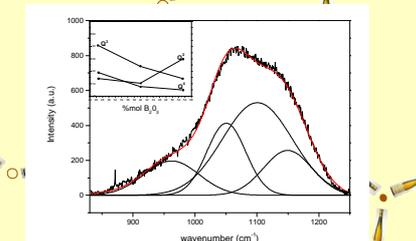
Curve fitted Raman spectra SBN53-20 of the spectral region between 800-1200 cm<sup>-1</sup>. Q<sup>n</sup> denotes a tetrahedral site, SiO<sub>4</sub> where n is the number of bridging oxygen per tetrahedron.
