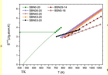
Configurational entropy of borosilicate melts against temperature. △ and ▲ correspond to data from Y. Linard [1].
