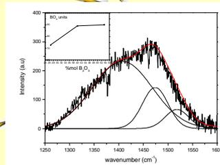
Curve fitted Raman spectra of the borosilicate glass SBN53-20 of the spectral region between 1200-1600 cm<sup>-1</sup>.
