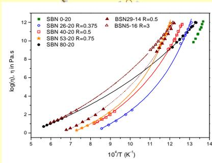
Viscosity of molten borosilicate as a function of 1/T. At low viscosity, measurements were made at CEA Marcoule for SBN40-20 and SBN26-20 and at IPGP for other melts. △ and ▲ are data from Y. Linard [1].
