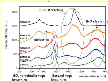
Comparison of Raman spectra of the five borosilicate glasses with constant Na<sub>2</sub>O content. The spectra have been measured at IPGP (Jussieu) at room temperature and  $\lambda = 488\text{nm}$ .
