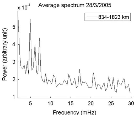
**Fig. 5.** Spectrum of the Doppler time series averaged for ranges between 834 km and 1823 km, for the time interval 18:12–18:48 UT. The intermediate zone, for ranges between 1150 km and 1400 km, where the  $S/N$  ratio is too low, has been excluded from the average. The horizontal frequency scale extends from 2 to 30 mHz. The strongest peaks are observed between 3 mHz and 8 mHz. Weaker peaks are observed at larger frequencies, up to 30 mHz.
