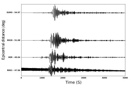
**Figure 3.** Seismograms corresponding to the event that occurred in Pakistan M = 7.7 (24 September 2013) that were recorded by the French INSU OBS RR28 station, the German DEPAS OBS RR01 station, the Geoscope RER land station (La Réunion Island), and the temporary EURO land station deployed on Europa island in Mozambique Channel.
