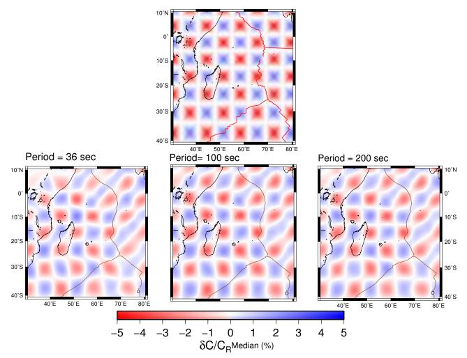
**Figure S1.** Checkerboard test of phase velocity, showing the reliability of the ray coverage of the area. Top: The input model. Bottom: The *Regionalization* map results for the 50, 100, 200 s periods.
