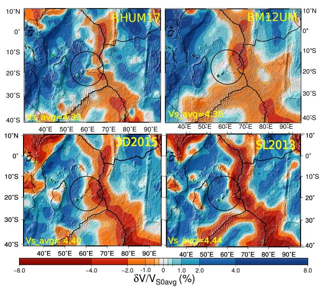
**Figure S12.** Comparison of shear velocity perturbation between the present model RHUM17 and the three recent global models, BM12UM, SL2013sv, and 3D2015 at 50 km in depth. Black circles indicate the area where model RHUM17 shows the shallow signature of a 'pipe-flow' connecting the La Réunion hotspot with the CIR, which is not resolved by the global models.
