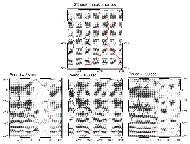
**Figure S4.** Checkerboard test of azimuthal anisotropy from the group velocity measurements, showing the reliability of the ray coverage of the area. Top: The input model. Bottom: The *Regionalization* map results for the 36, 100, 200 s periods.
