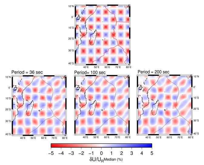
**Figure S3.** Checkerboard test of group velocity, showing the reliability of the ray coverage of the area. Top: The input model. Bottom: The *Regionalization* map results for the 50, 100, 200 s periods.
