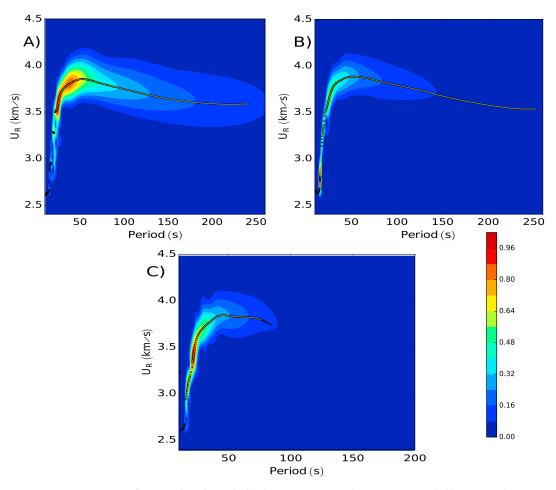
**Figure 6.** Dispersion curves for an earthquake in Thailand  $M = 6.8 \, 11$  November 2012, as recorded by (a) RER, (b) RR40, and (c) RR01. The colored backgrounds indicate the time frequency signal amplitudes, with red-based colors as the largest amplitudes. The yellow lines show the manually picked dispersion curves. The measured period range is broader for RER and RR40 than for RR01 due to the different sensors in the stations.
