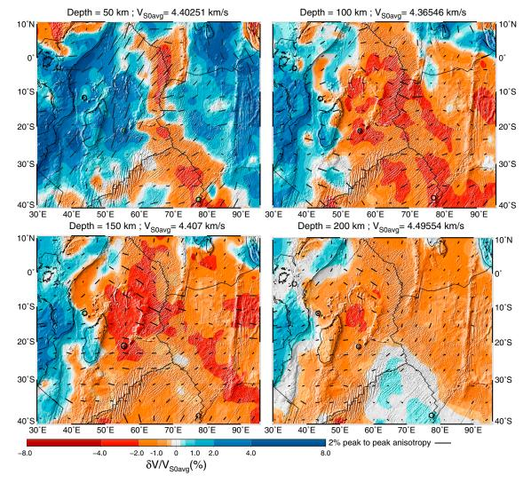
**Figure 8.** *S<sub>V</sub>* wave velocity perturbation with respect to the mean velocity at the different depths of 50, 100, 150, and 200 km. Fast anisotropy directions are plotted with bars, where the strength is normalized with respect to the maximum value at each depth. Black circles indicate the hot spot locations in the area.
