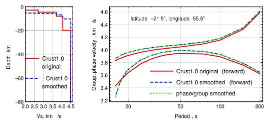
Figure S8. Crustal analysis for the grid point lat. -21.5, lon. 55.5. Left: The one-dimensional  $V_s$  models for the inversion of the original Crust1.0, and the smoothed version. The  $V_s$  values are not inverted due to the period range of the inversion (16 s to 240 s) that only allows evaluation of the thicknesses of the layers. Right: The phase and group velocity results for the original (red line) and the smoothed version of Crust 1.0.
