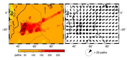
**Figure 7.** Data set used in the group velocity calculation. (left) Density path map. (right) Azimuthal coverage of the area, where the number of paths per unit area  $(2^{\circ} \times 2^{\circ}$  cell) are binned in the azimuth range of 30°, and the vectors are saturated at 20 paths. There is higher density of paths beneath Réunion and the central/eastern part of the map than beneath Africa; the path coverage is redundant everywhere.
