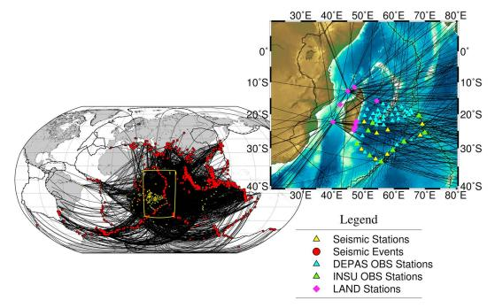
**Figure 2.** Global distribution of the ~300 earthquakes sources (red) and 130 stations (yellow) used in this study. Black lines show the great circle paths. The magnified panel (right) shows the distribution of the RHUM-RUM stations and the final raypath coverage used in the procedure.
