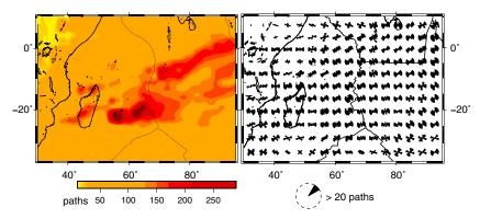
**Figure 4.** Data set used in the phase velocity calculation. (left) Density path map. (right) Azimuthal coverage of the area, where the number of paths per unit area  $(2^{\circ} \times 2^{\circ}$  cell) is binned in the azimuth range of 30°, and the vectors are saturated at 20 paths. However, the density path beneath Réunion and the central/eastern part of the map is higher than beneath Africa. The path coverage is redundant everywhere.
