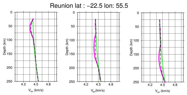
**Figure S6.** The synthetic (magenta) and inverted (black-dots) S-wave velocity models. The smooth anomaly is placed at different depths, and it is always well recovered.
