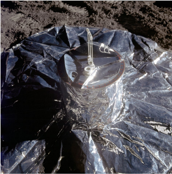
Figure 1. Gnomon used on the Moon with the passive seismic experiment (PSE) during the Apollo 14 mission.
