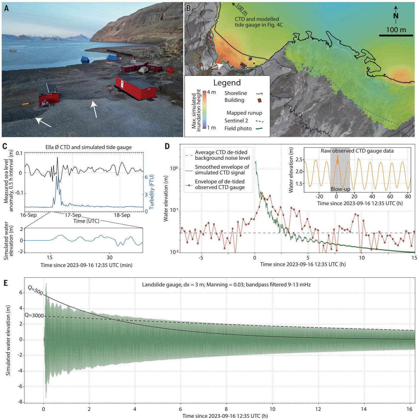
**Fig. 4. Tsunami observations and modeling.** (A) Drone photo looking east-northeast showing the 4-m runup height at Ella Ø (white arrows) [Source: Joint Arctic Command/Sirius of the Danish Navy]. (B) Mapped and simulated tsunami runup at Ella Ø. (C) Observed and simulated tsunami at Ella Ø using the GloBouss tsunami model (43) (Fig. 1C). (Top) Sea level and turbidity from the conductivity, temperature, and depth (CTD) station. FTU, formazin turbidity
