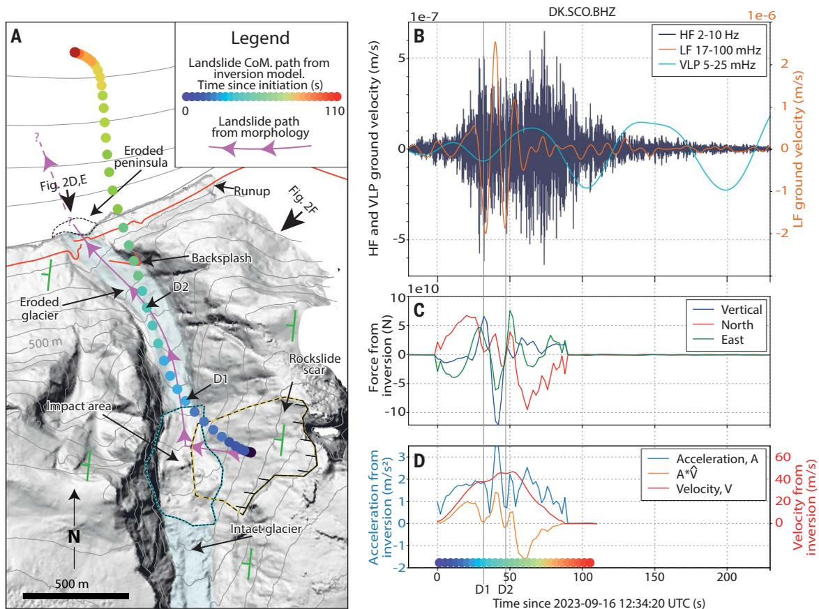
**Fig. 3. Landslide seismic signal and modeling.** (A) Geomorphological map showing the landslide center-of-mass (CoM) runout paths from morphological interpretation and seismic inversion. Green symbols indicate the strike and dip direction of the foliation. (B) The seismic signal recorded at DK.SCO.BHZ (313-km distance), shifted by the travel time between the source location and the station (at 3 km/s velocity), with different bandpass filters applied.
