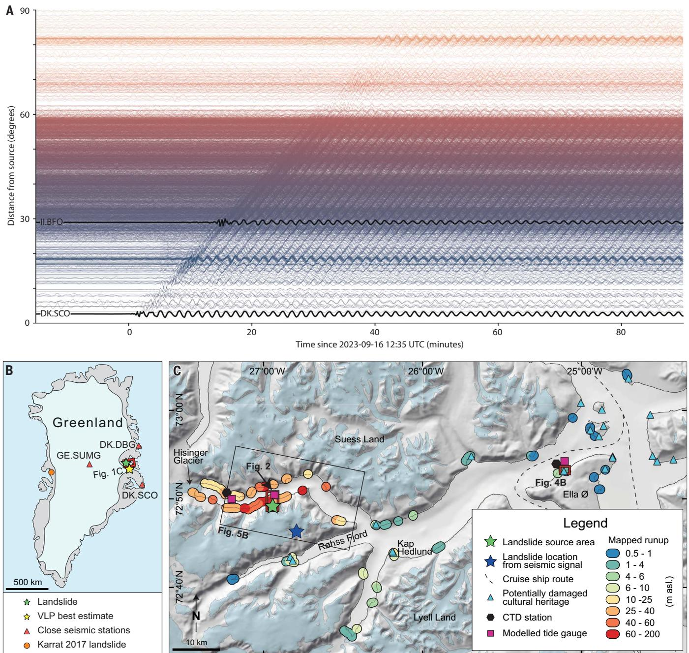
**Fig. 1. Seismic signal, position, and local setting.** (A) Record section showing vertical-component waveforms from ~4,500 seismic stations up to 90° (10,000 km) from Dickson Fjord, with data bandpass filtered at 25 to 115 s and waveforms colored by epicentral distance. Based on the move-out with a phase velocity of 4.1 km/s, these waves can be identified as Rayleigh waves. Stations DK.SCO and II.BFO are highlighted, with detailed views of their waveforms shown in
