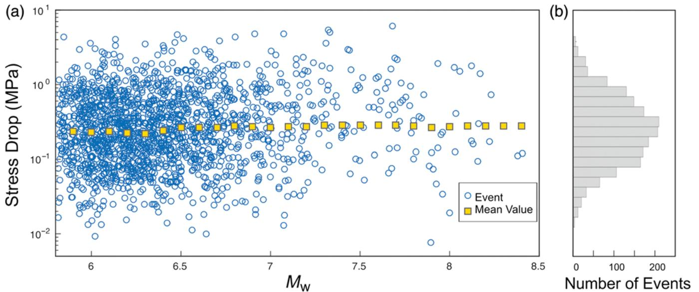
▲ **Figure 4.** (a) Stress-drop values (MPa) obtained from the SCARDEC catalog of STF for shallow earthquakes (depth < 35 km) using equation (4) for  $k = 0.32$  (value for  $P$  waves in the Madariaga, 1976, model),  $V_S = 3900$  m/s and  $f_c = 0.6/T$ . Mean values are computed for bins of  $M_w \pm 0.1$ . (b) Distribution of  $\log_{10}(\Delta\sigma)$ . The color version of this figure is available only in the electronic edition.
