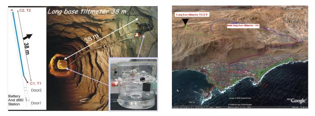
One component of a long base inclinometer has been installed in August 2007 in a tunnel of the Neuquen mine 10 km NNE of Iquique. The instrument was developed by F. Boudin (IR Geosciences Montpellier). A second component will be installed by the end of this year.
